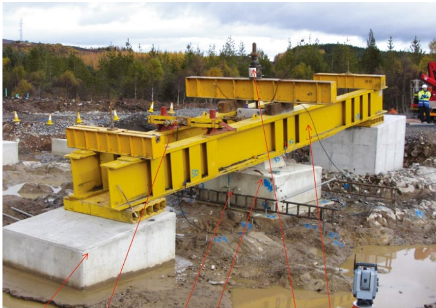
Reaction pad Hydraulic jack for horizontal shears Test foundation Displacement gauges Test beams Hydraulic jack for axial leg loads
