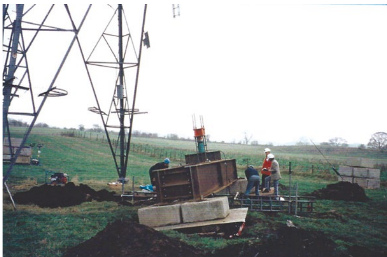
Figure 13.43 Full-scale testing of an existing foundation – support in-situ. (Note: Bottom tower leg disconnected and removed during the test)
