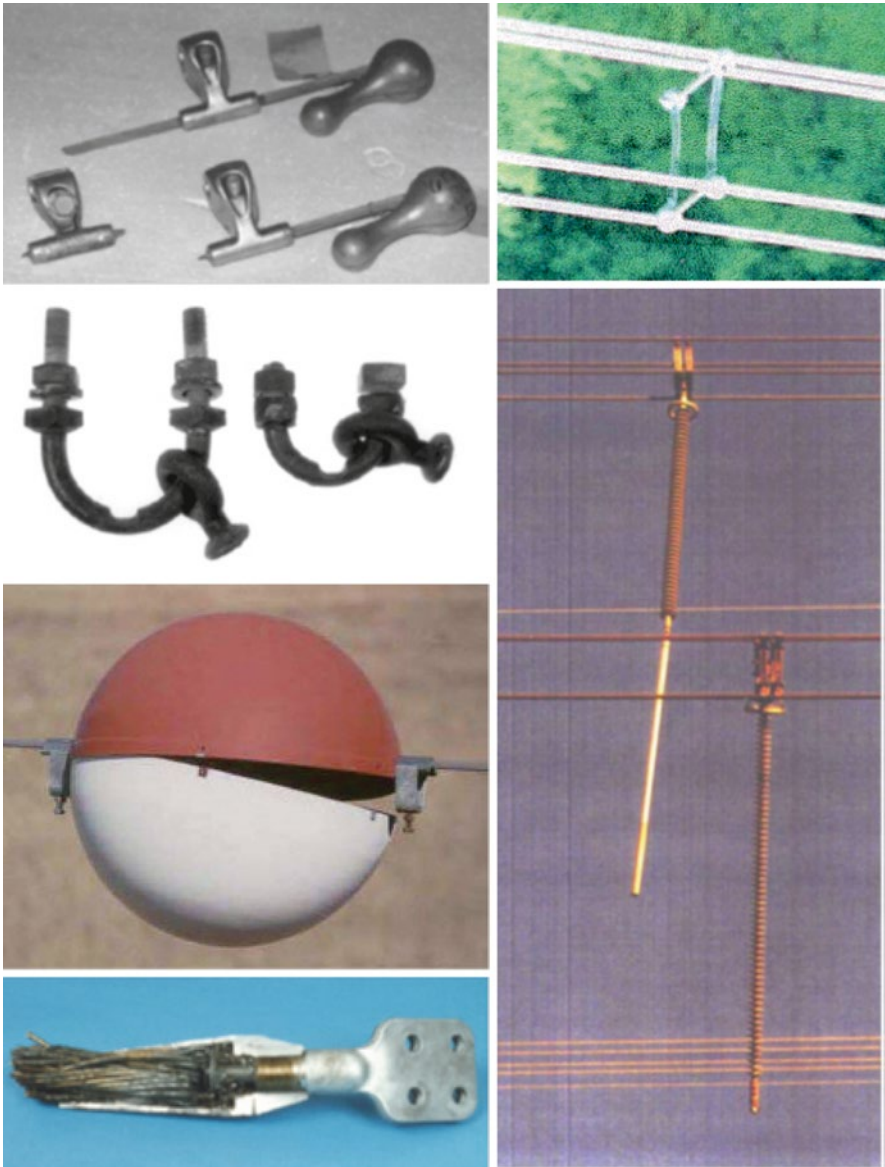
Figure 9.20 Samples of deteriorated hardware. Clockwise from top left : Aeolian Vibration Dampers, Quad Bundle Spacer, Interphase Spacer, Conductor Compression Fitting, Aircraft Warning Marker, Suspension String “U” and “Eye” Bolts.
