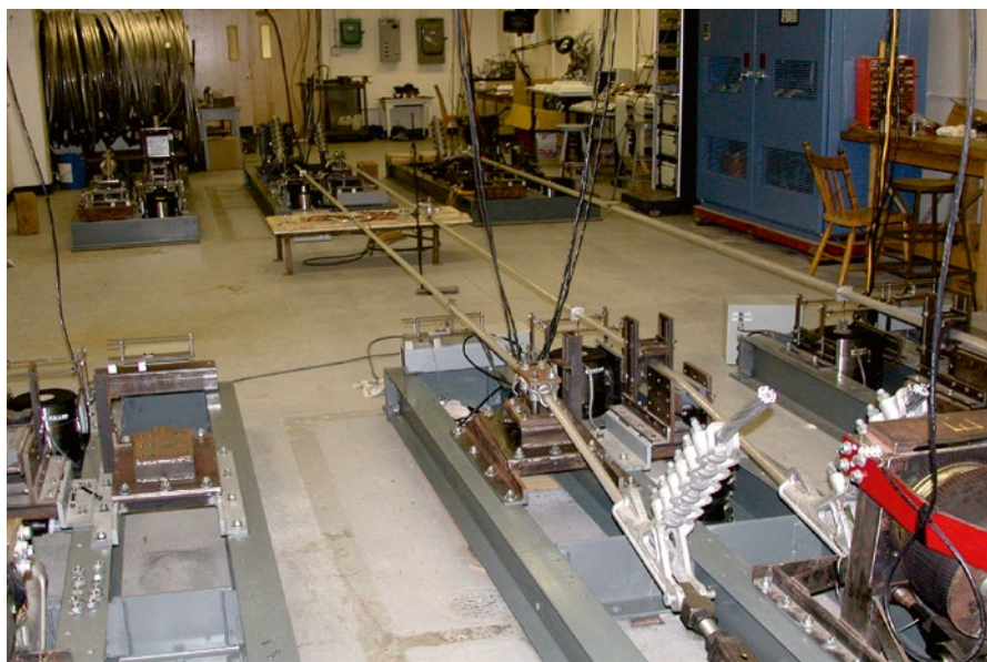
Figure 10.29 Resonance type test benches, GREMCA's laboratories.
