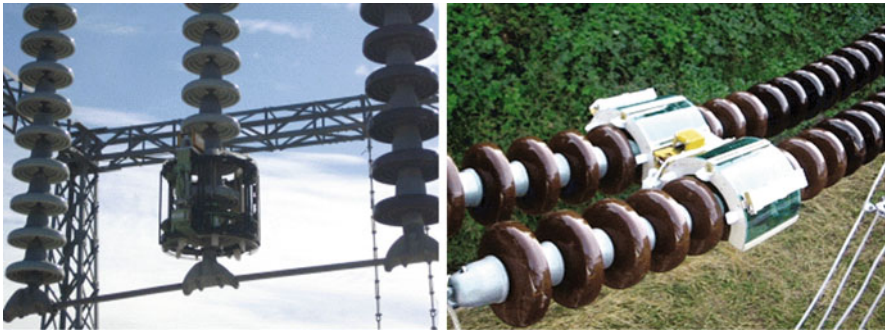
Figure 16.20 Live-line insulator cleaning robot developed by KEPCO 2006.
