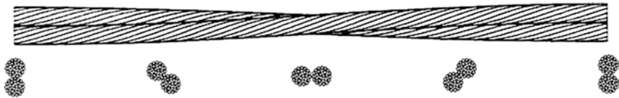
Figure 8.14 Twisted Pair conductor which consists of two conventional conductors wrapped helically about each other with a lay length on the order of 3 meters.
