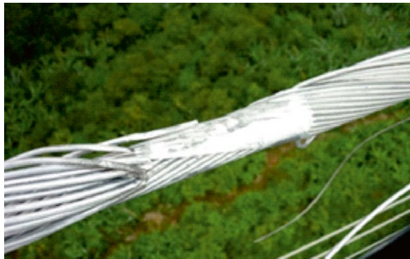
Figure 9.76 Damper displaced towards the span center on ground wire.
