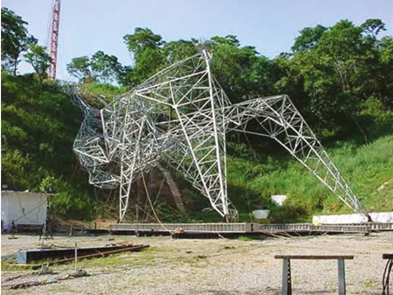
Figure 12.58 Destructive test – 500 kV TL Tower.
