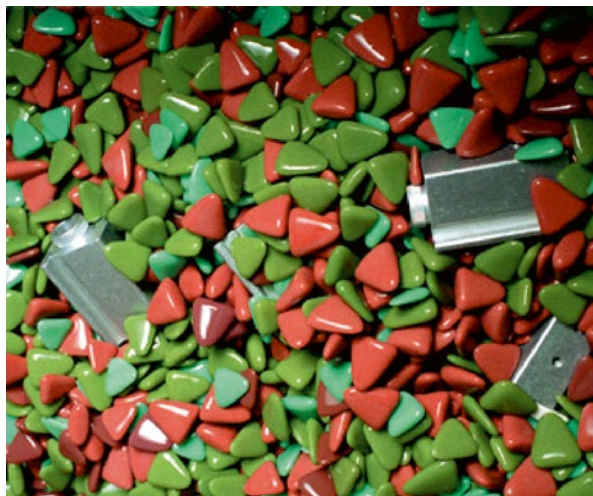
Figure 9.4 Aluminium pieces and abrasive pellets inside the tumbler.
