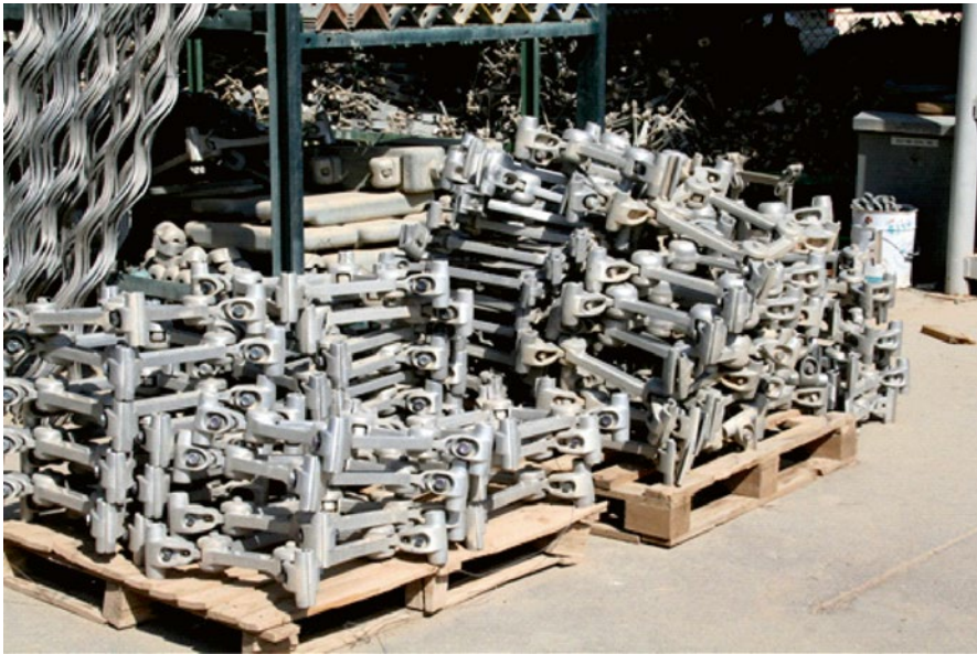
Figure 9.27 Spacer dampers and other fittings stacked in the construction camp yard.
