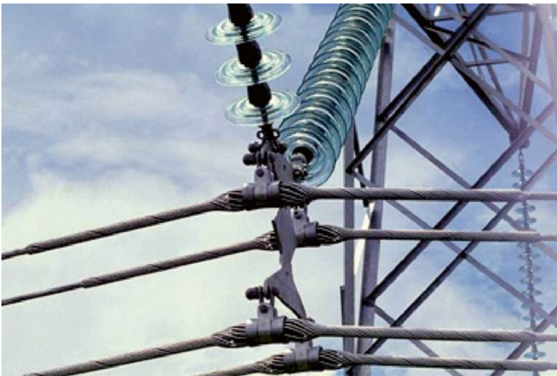
Figure 9.49 HAES suspension clamps.
