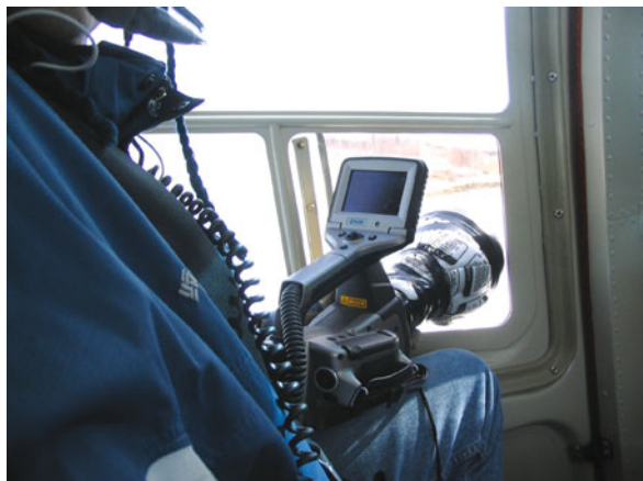
Figure 16.5 Thermographic inspection performed from a helicopter.
