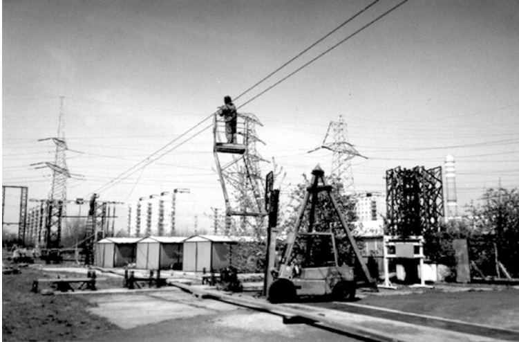
Figure 10.82 Test arrangement applying short circuits to a 60-m span length with one spacer at mid-span (Lilien and Papailiou 2000).
