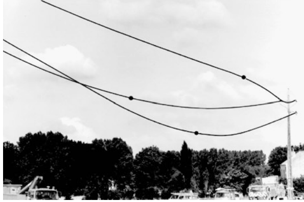
Figure 10.79 Instantaneous position of the conductors taken during three-phase short-circuit test on 15-kV distribution line near Liège (Lilien and Vercheval 1987).
