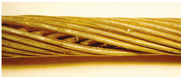
Figure 16.2 Broken Inner Conductors Strands.
