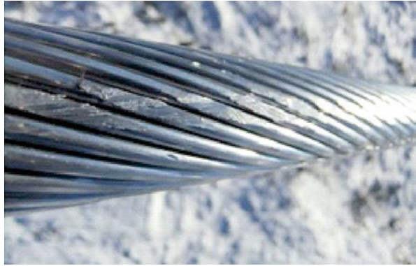
Figure 9.127 Aluminium damage caused by cable reel during stringing.
