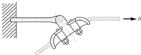
Figure 9.24 Typical tension fitting test (Splice shown, but not required for tension fitting test).
