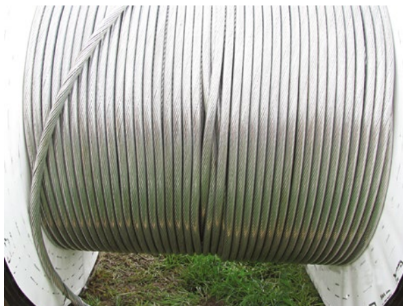
Figure 15.34 Conductor Pull-Down due to excessive braking force on the payoff (Courtesy of Southwire Co.)
