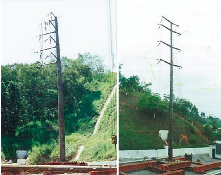
Figure 12.35 Pole deflections during Tests.
