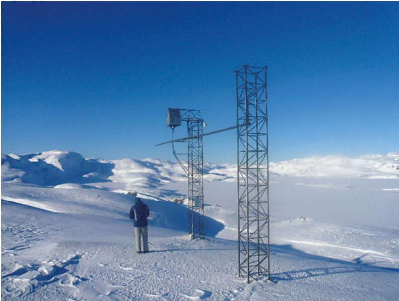
Figure 7.21 Rack for measuring rime icing in Norway (Photo: B.E.K. Nygaard).
