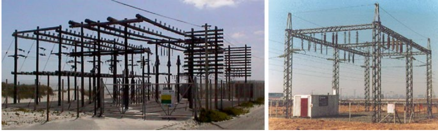
Figure 11.14 Permanent insulator research stations at Koeberg and Sasolburg, South Africa (Cigré WG B2.03 2007).
