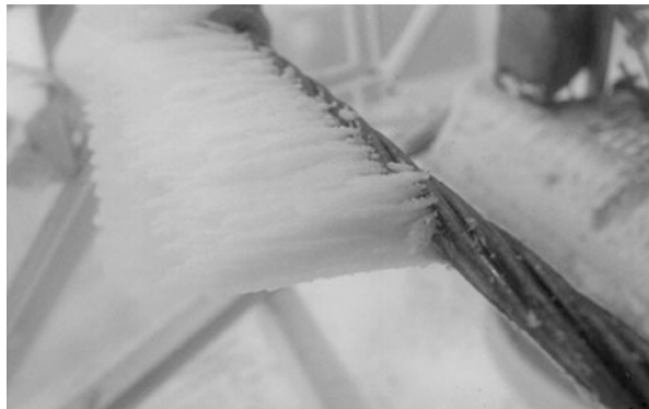
Figure 7.15 Rime icing vane (Wareing 1999).
