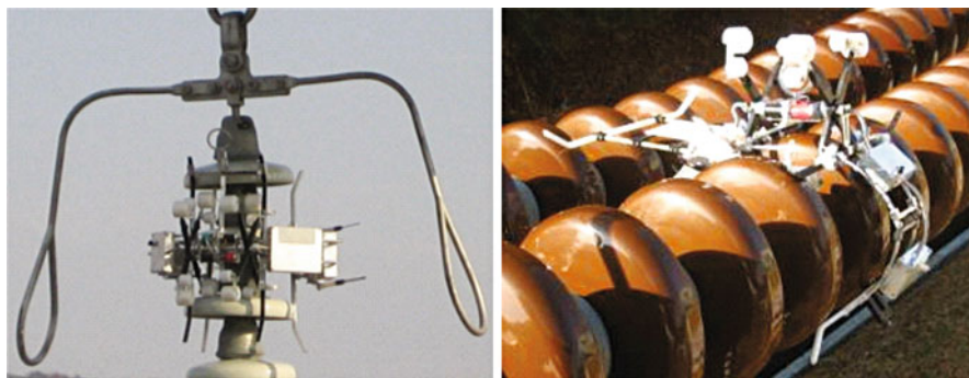
Figure 16.21 Live-line insulator inspection robot developed by KEPCO, 2010.
