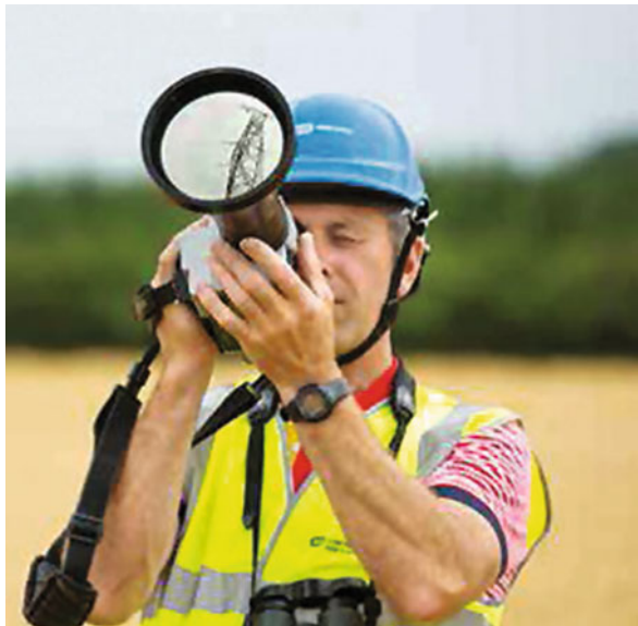
Figure 16.4 Thermographic inspection performed from the ground.
