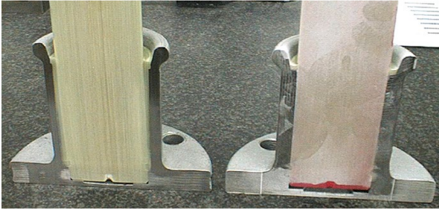
Figure 11.63 Post insulator dissected, no cracks, “test passed”: left half without dye, right half with dye (Papailiou and Schmuck 2012).
