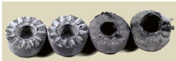
Figure 9.97 Damaged spacer-damper elastomer element.
