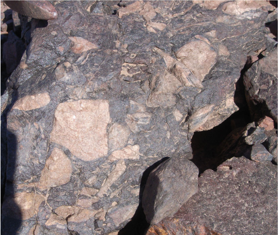
Fig. 10 Conglomerate of Seyala Conglomerate Formation in outcrop east of Rouessa open pit. Light clasts are quartzite; dark matrix is a fine-grained mixture of iron
