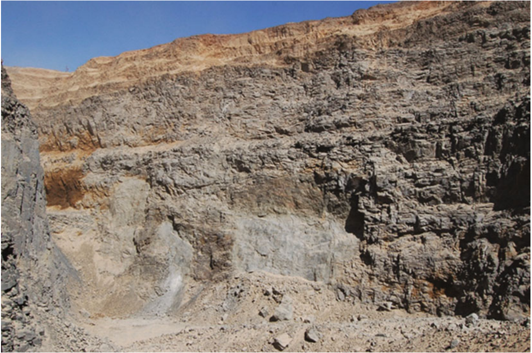
Fig. 18 Northeast wall of Guelb El Rhein open pit. Note prominent orange oxidized zone extending downward approximately 30–50 m from surface. Height of pit wall is ca. 200 m. USGS photo
