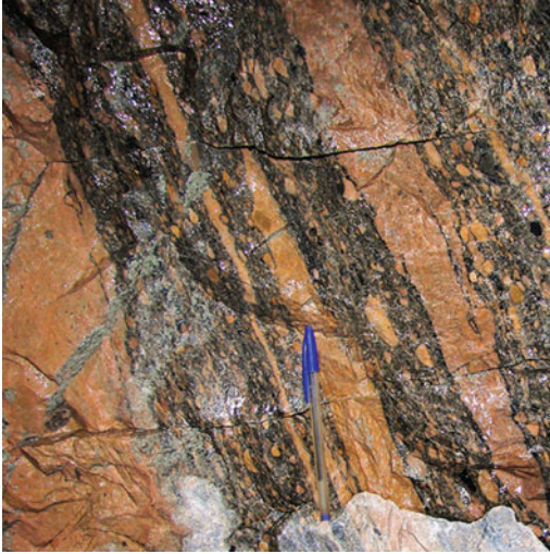
Fig. 3 Photograph of brittle-ductile deformation along Yalea Shear with gold mineralization hosted in dark matrix of pink albite-ankerite hydrothermal breccia (Lawrence et al. 2013a)
