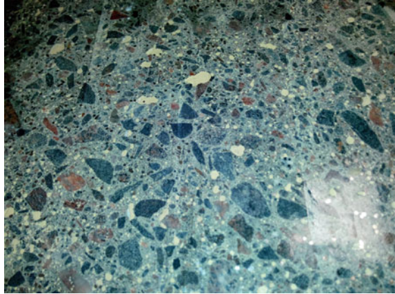
Fig. 1 A cut through SFRC, the white parts are filled pores, the silvery-bright spots are cut fibres
