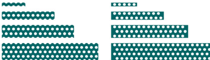
Fig. 6 Representation of beam samples of increasing size generated by finite element meshes shown in Figs. 5 (right) and 7 (left)
