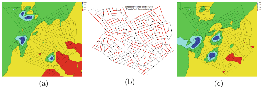
Fig. 5. (a) Total head of system (m) prediction by EPANET hydraulic simulation in Fig. 4(a); (b) MC identification of failed pipes within the network; (c) Total Head of System (m) considering the effects of the NOPB risk factor as described in Fig. 4(b) (color figure online).
