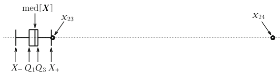
Fig. 7.7 Box diagram used to identify outlier candidates. Outliers may be expected outside of the interval [X_-, X_+] = [Q_1 - \frac{3}{2} \text{IQR}, Q_3 + \frac{3}{2} \text{IQR}]
