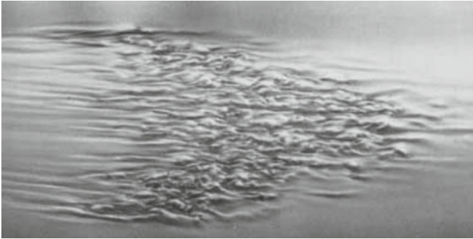
Fig. 3.11 Visualization of a turbulent spot in a boundary layer as seen from above. This is representative of a perturbation that developed from a Tollmien–Schlichting instability. The fluid flow is from left to right , but the spot develops in the upstream direction (i.e., to the left ). From: Cantwell et al. (1978)
