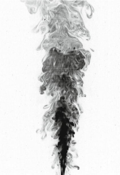
Fig. 6.23 a Visualization of a submerged round free jet with a Reynolds number of 2 \times 10^3 . The jet is issued from 1 mm diameter nozzle, and the displayed image height corresponds to 45 mm. Image taken by: Fukushima et al. (2002). b Photograph of the exhaust plume of a TITAN IV rocket discharging upward during a ground-based test. The bright plume is approximately 120 m high atop a 30 m test stand. The Reynolds number is about 2 \times 10^8 . Details are given by Mungal and Hollingsworth (1989). Use a compass or protractor to compare the jet spreading rates
