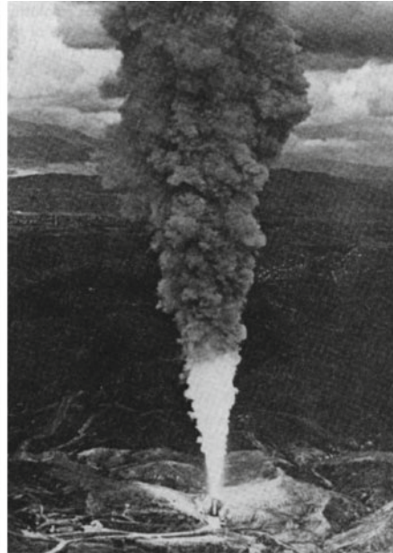
Fig. 6.23 a Visualization of a submerged round free jet with a Reynolds number of 2 \times 10^3 . The jet is issued from 1 mm diameter nozzle, and the displayed image height corresponds to 45 mm. Image taken by: Fukushima et al. (2002). b Photograph of the exhaust plume of a TITAN IV rocket discharging upward during a ground-based test. The bright plume is approximately 120 m high atop a 30 m test stand. The Reynolds number is about 2 \times 10^8 . Details are given by Mungal and Hollingsworth (1989). Use a compass or protractor to compare the jet spreading rates
