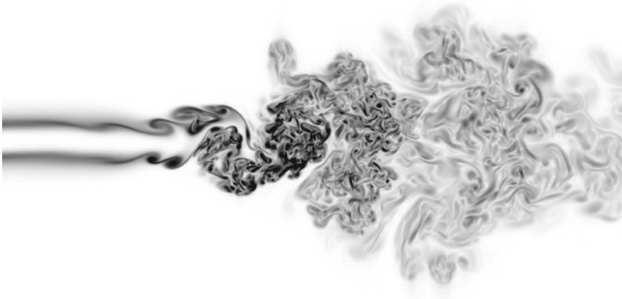
Fig. 6.18 Visualization of the vorticity magnitude of a round jet at Re = 3 \times 10^3 developing from laminar to turbulent flow. Notice the development of the shear layers in the laminar domain, akin the Kelvin–Helmholtz instability discussed in Sect. 3.2. Data are obtained from a direct numerical simulation (DNS) by Moore (2009)
