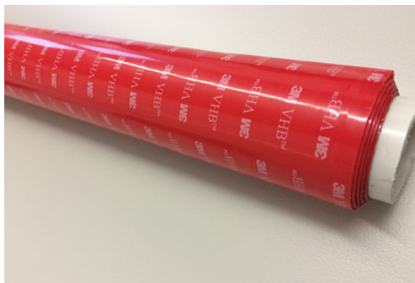
Fig. 1 3M VHB™ tape: a commonly used dielectric for DEAs (the tape is transparent, the backing is red)
