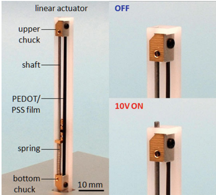
Fig. 19 Photographs of linear actuator utilizing PEDOT/PSS film (Reproduced from Okuzaki et al. (2013a))
