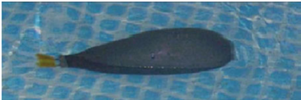
Fig. 7 WANDA the fish articulated with trilayer actuators and its caudal fin arrangement (Fay et al. 2010; Carpi et al. 2011). It must be noted that the body and caudal fin of WANDA have been optimized to minimize the drag and increase its swimming efficiency, compared to NEMO
