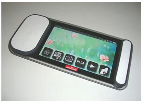
Fig. 10 Prototype deformation detection touch panel
