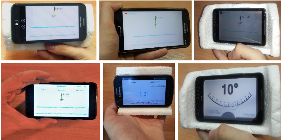
Fig. 2 – Various polystyrene extensions for smartphones with own or 3 rd -party scoliometer app
