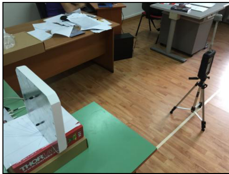
Fig. 4. Field emissions measurement of RFID system.
