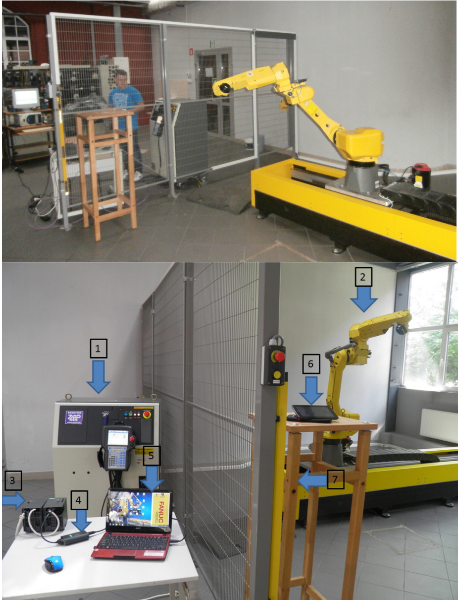
Fig. 2. Remote robot control stand. 1 robot controller, 2 industrial robot, 3 PLC controller, 4 communication adapter, 5 laptop, 6 tablet, 7 safety curtains [26]
