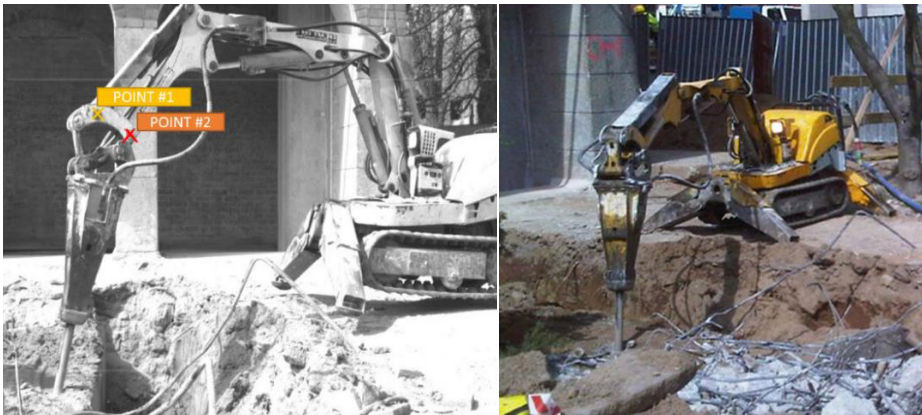
Fig. 4. Tracked points in TEMA Motion photogrammetric software – footage recorded by high-speed camera Phantom (left) and standard camera (right).
