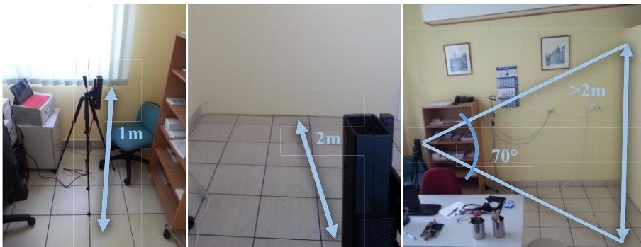
Fig. 1 – Kinect sensor position in the GP examination office illustrating its vertical FOV
