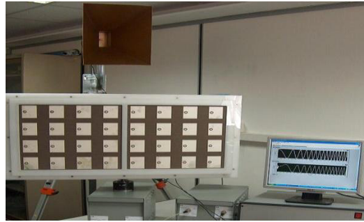
Fig. 3. Photograph of the complete L-band SDRadar system.
