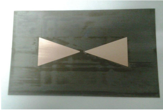
Fig. 5. Realized UHF butterfly antenna prototype.
