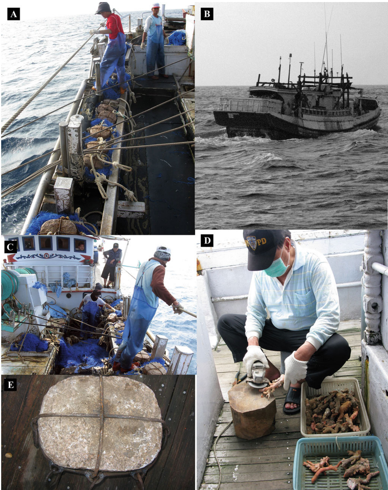
Fig. 46.9 Taiwanese fisheries. (a) Tangle nets are still the only fishing tackle used to collect precious corals in Taiwan. Each tangle net is composed of one big stone (e) used to sink the net and up to seven pieces of net. Windlasses are used to release and manipulate tangle nets. (b) Precious coral fishing vessel. Most of the fishing vessels are smaller than 50 tons, but vessels of up to 100 tons can be used for coral fishing. All vessels must be equipped with VMS (Fishing Vessels Monitoring System). (c) Each fishing vessel has four workers, one captain, and one
