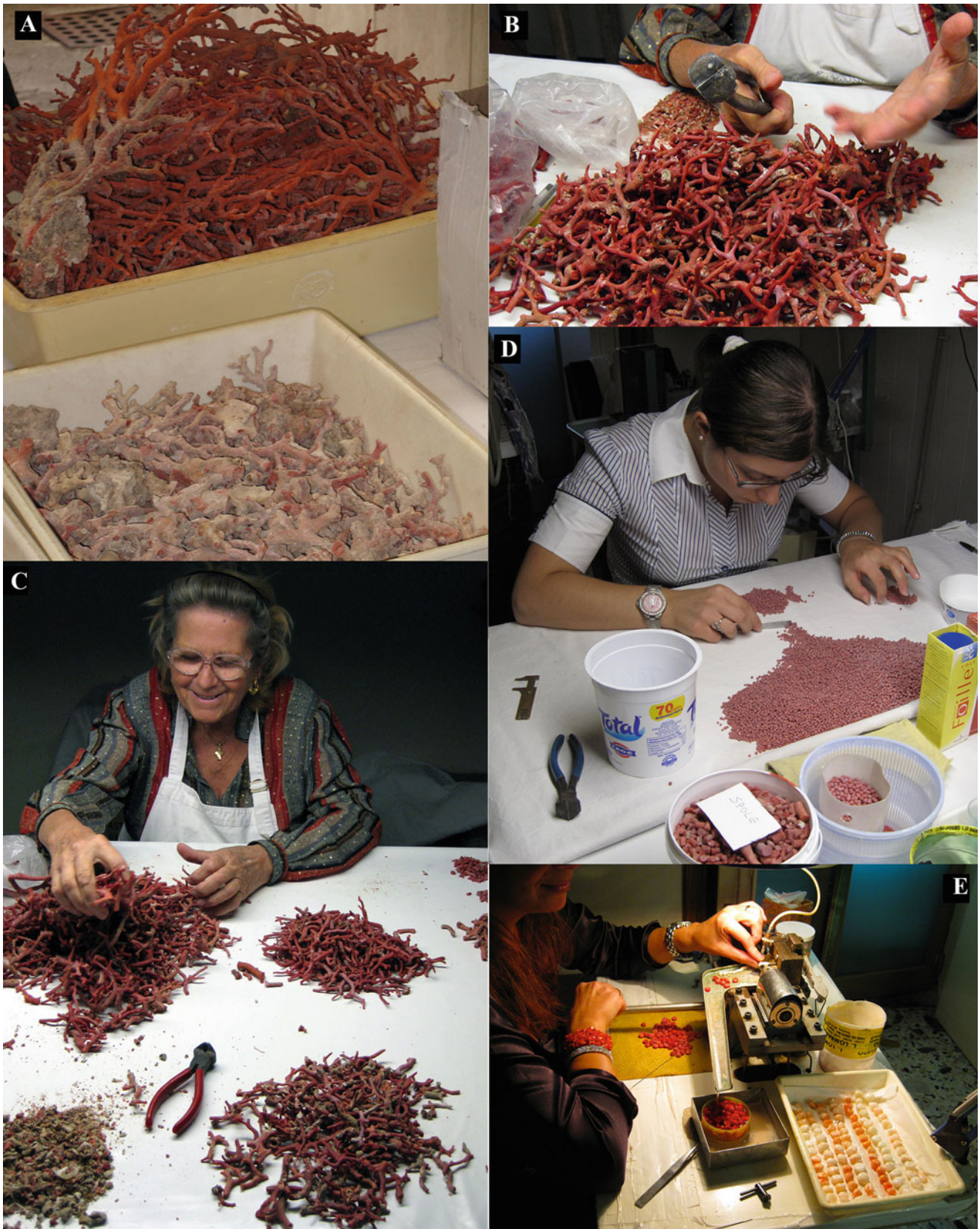
Fig. 46.7 Processing of Corallium in Torro de Greco, Italy. Common lapidary techniques are used to cut, grind and polish precious corals. In some cases the carves pieces and beads are soaked in a solution of hot
