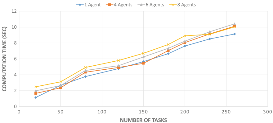
Fig. 9 Computation time for clustering imitation algorithm with different number of agents and tasks; because each robot executes each clusters tasks in parallel with other robots, MMP with clustering overcome the algorithm without clustering in total algorithm time in all cases
