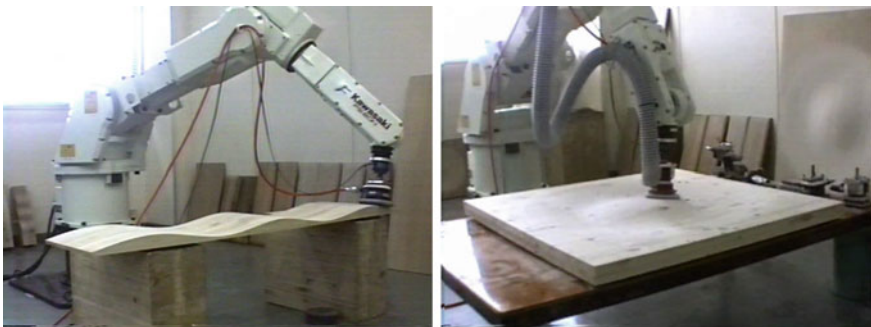
Fig. 3 Robot sander for wooden workpieces developed based on FS20 provided by Kawasaki Heavy Industries, LTD., in 2000
