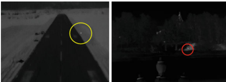
Fig. 2 Left 30 W NIR led lamp near runway visible through narrow-band IR filter in sunny day from 350 m; Right 20-cm object heated by portable gas burner is visible from 700 m distance on thermal camera image in daylight conditions
