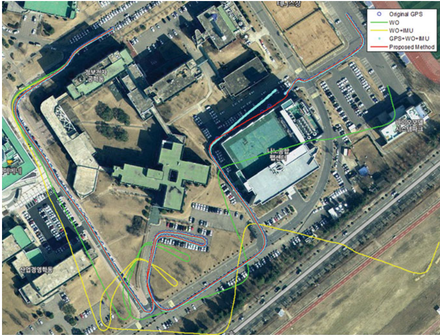
Fig. 7 Experiment results. The blue circle means the pose from GPS, the green solid line WO, the yellow solid line WO + IMU, the light blue dot GPS + WO + IMU, and the red solid line proposed method
