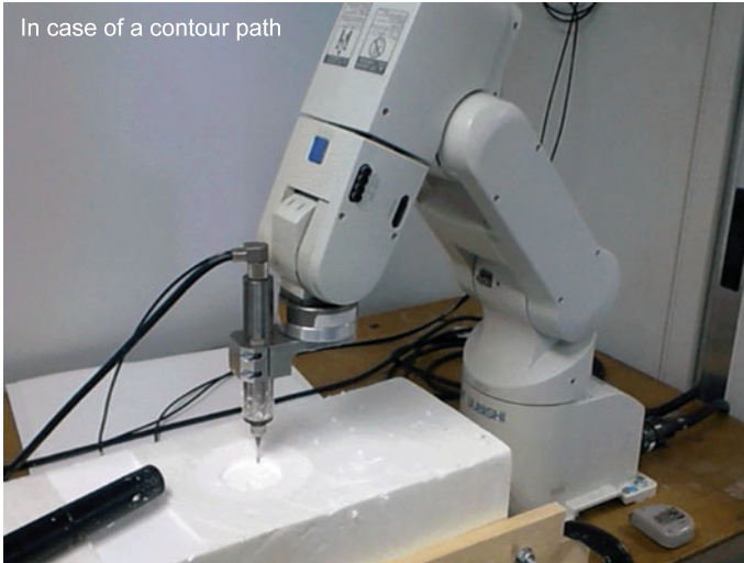
Fig. 6 Machining robot being developed based on a small industrial robot RV1A provided by Mitsubishi Electric Corp. in 2015
