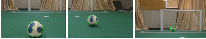
Fig. 2 From left to right , it is shown that the ball is detected for near, mid-, and far distances
