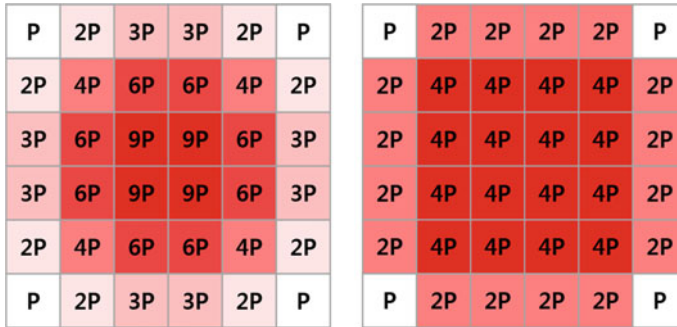
Fig. 3 In a feature map, the probability for selection varies according to the location. Left \beta = 2 ; Right \beta = 3
