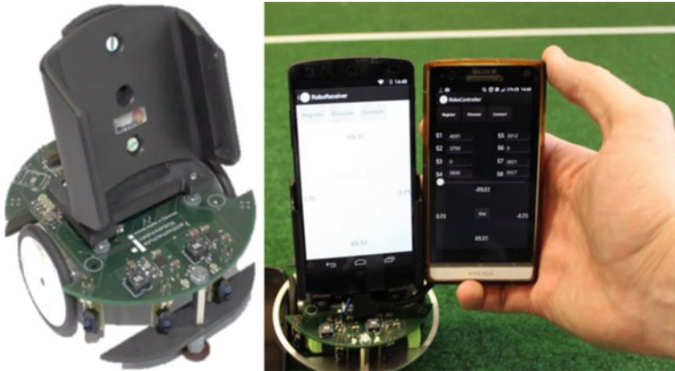
Fig. 2 Smartphone integration into the robot platform via a standard socket ( left ) and wireless remote access for system setup and data recording via Wi-Fi or Bluetooth ( right )
