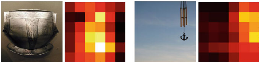
Fig. 1 Feature maps in the mid-level and high-level layers of CNNs use information from the inferior locations of original images. Left a good example of an image containing a large centered object and its corresponding feature map at the top of the network before global average pooling; Right a bad example of an image containing a small side-positioned object and its corresponding feature map
