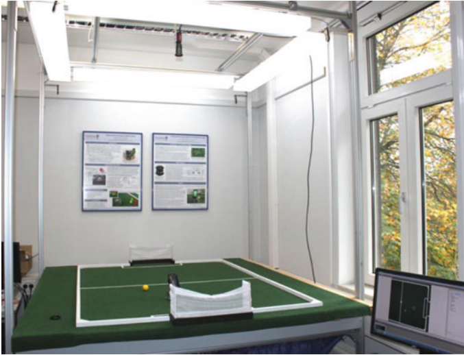
Fig. 3 Tele-workbench platform with video recording option (camera located over the field, live video displayed and recorded at PC, and robot data optionally included)
