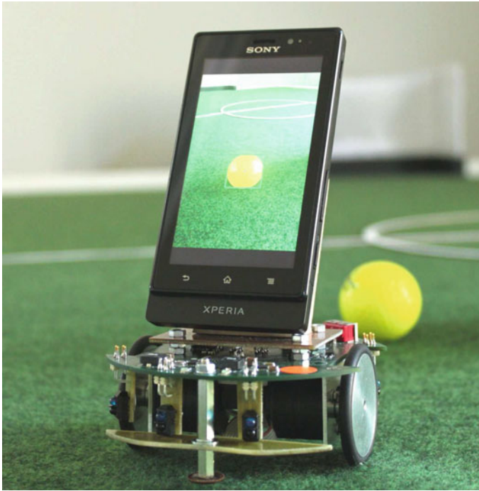
Fig. 1 The Zorro robot consisting of the mobility module and a smartphone
