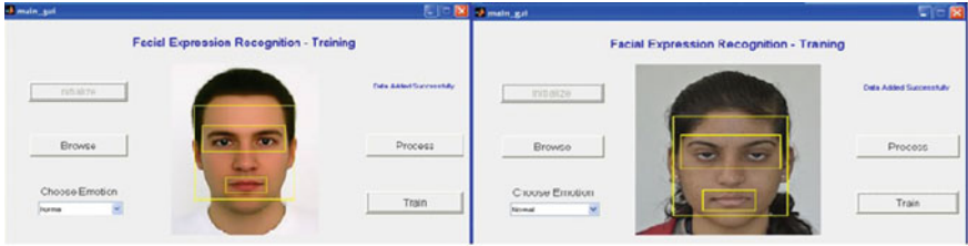
Fig. 4 Face detection, localization of lip and eye region for bmp and jpeg images
