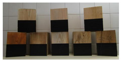
**Fig. 4.** The eight lumber samples used in the experimental tests (exposed side/side with black tape insulating).
