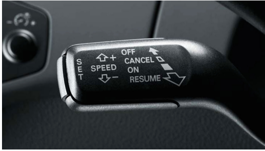
Fig. 1. Function buttons on the control lever of a cruise control system. (The figure is from the home page of Audi.)
