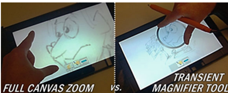
Fig. 3.11 Pinching with the nonpreferred hand zooms the full canvas, while a preferred hand pinch with the pen-in-hand brings up the transient magnifier tool. In this way we support a new class of multi-touch gesture which incorporates the context of which hand produces the touch as well as whether (and how) the pen is being gripped at the time of the touchscreen contact. Image © Ken Hinckley, 2014. Used by permission. All rights reserved
