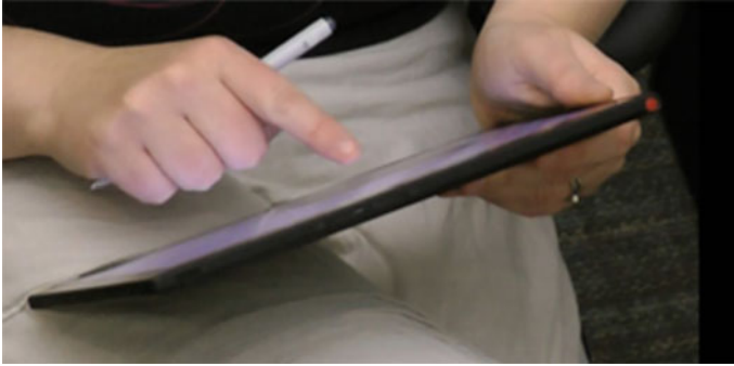
Fig. 3.4 What input modality is this? At first glance one might dismiss this as a straightforward illustration of a ‘touch’ interaction—a user about to put his index finger to the touchscreen. But a more careful look at the oft seen, but seldom noticed details of how the participant is using the tablet, and the stylus, with both hands suggests that the answer is not so simple. Photo © Ken Hinckley, 2014. Used by permission. All rights reserved
