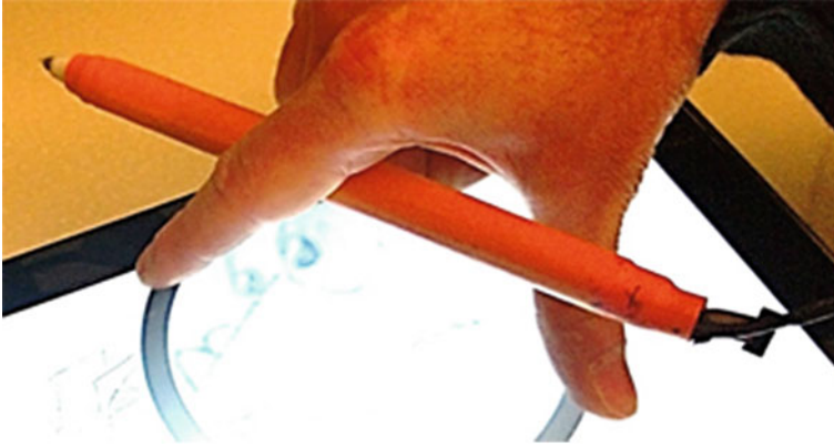
Fig. 3.7 Augmented stylus prototype in action. The current prototype is tethered, and somewhat bulky, but not so much so that it precludes interactions such as touching the screen while the pen is tucked between the fingers. Photo © Ken Hinckley, 2014. Used by permission. All rights reserved
