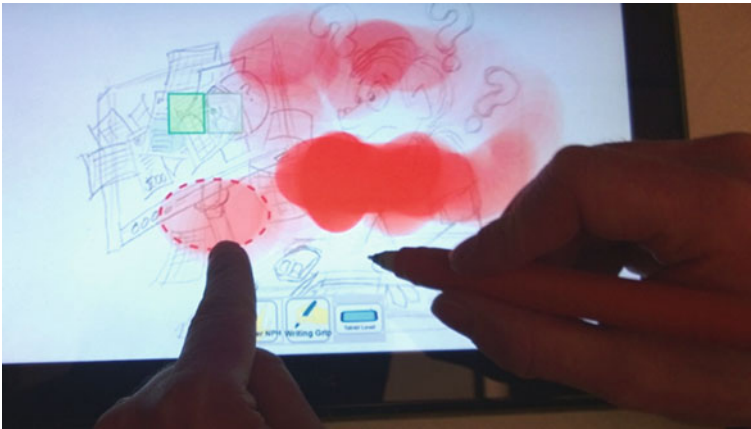
Fig. 3.12 The airbrush tool. A touch from the nonpreferred hand indicates where to airbrush, while the preferred hand orients the pen in 3D to control the conic section of the resulting spray. Note that the pen does not have to stay “within range” of the traditional 1 cm sensing range of the tablet digitizer during this interaction, because our augmented sensors provide the 3D orientation information. Photo © Ken Hinckley, 2014. Used by permission. All rights reserved
