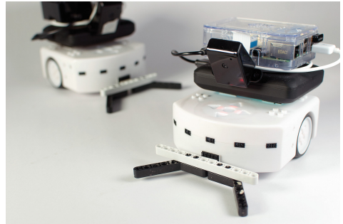
Fig. 1. Thymio II robot, developed by The École Polytechnique Fédérale de Lausanne (EPFL) and École Cantonal d'Arts de Lausanne (ÉCAL), with Raspberry Pi 2, Raspberry Pi NoIR camera, WiFi dongle, external battery and a LEGO gripper.
