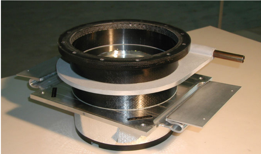
Fig. 3.14 Glassfibre-reinforced epoxy support post (CERN photo)
