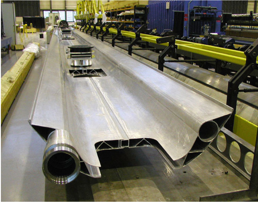
Fig. 3.10 Extruded aluminium alloy (A6060) bottom tray of cryostat thermal shield (CERN photo)
