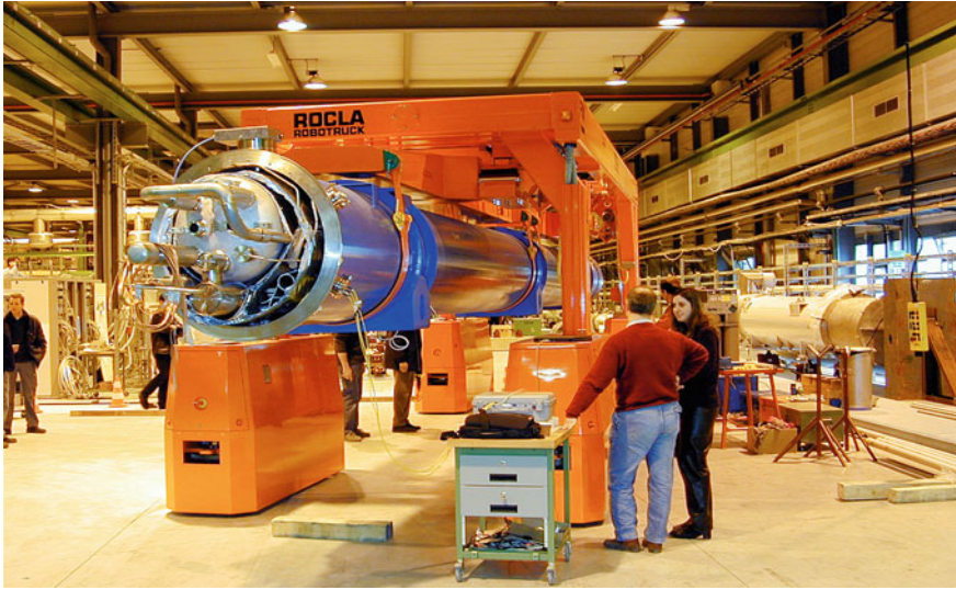
Fig. 3.17 Completed dipole cryo-magnet transported to test hall (CERN photo)
