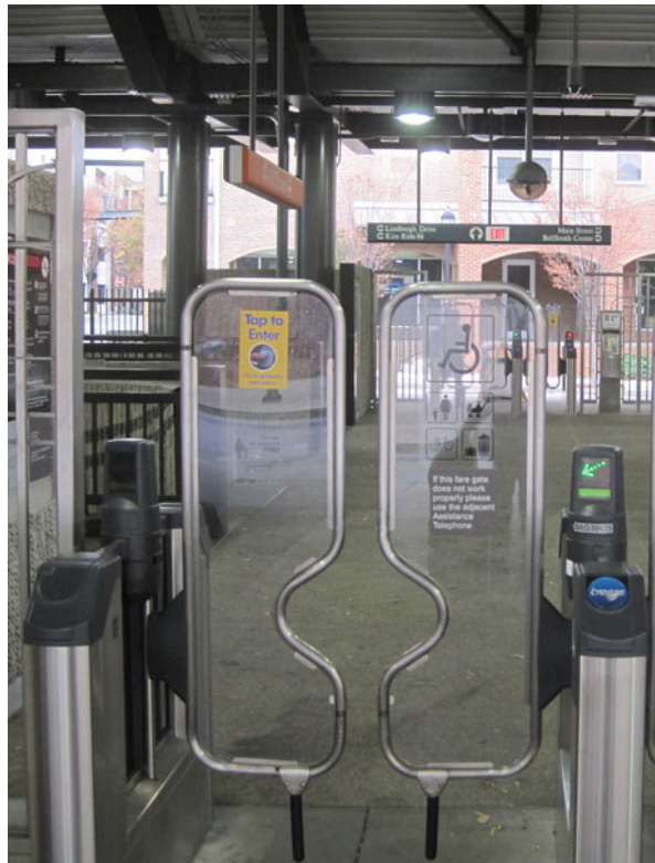
Fig. 5.5 Flexibility is provided by physical or digital interfaces, such as large entry-crossing tap-to-enter “buttons” that do not require precision (Photo: Jon A. Sanford)
