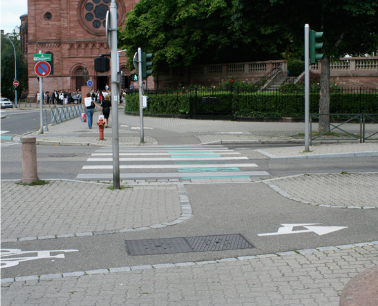
Fig. 5.3 Whereas specialized design uses signage to indicate a design element is for someone with a disability, universal design is everyday design intended for everyone, such as a crossing where all modes of transportation (foot with or without a long cane, wheeled mobility aid, bicycle, motor vehicle) are integrated (Photo: Jon A. Sanford)
