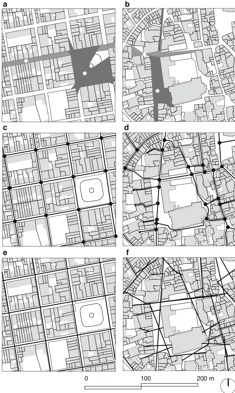
Fig. 3.1 A brief introduction to syntactic representations. On the left , the center of the planned Bastide de Mirande, Gascogne, France; on the right , the historically evolved center of Carpentras, Vaucluse, France. (a, b) 'Isovist' or 'visibility' polygons drawn from two selected locations in each city; (c, d) Center line maps for each city. Larger black circles represent street intersections offering navigation choices. Small black circles represent dead ends. (e, f) 'Fewest lines' maps for each city
