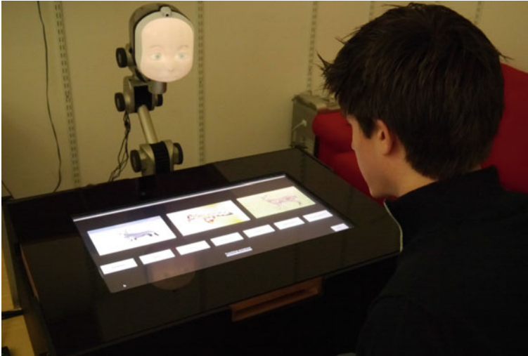
Fig. 5.6 Experimental setup, with the social robot sitting across the participant. The participant is invited to teach the robot to correctly match images of animals with animal classes
