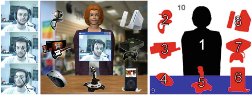
Fig. 4.7 A scenario involving a virtual agent and several objects. The user's gaze behaviour ( left ) is tracked as the agent conducts gaze behaviours towards various objects ( centre ). Gaze and attentive behaviours towards specific elements of the scene are recorded in real-time through Virtual Attention Objects ( right ) as a basis for monitoring user engagement in the scenario [21]
