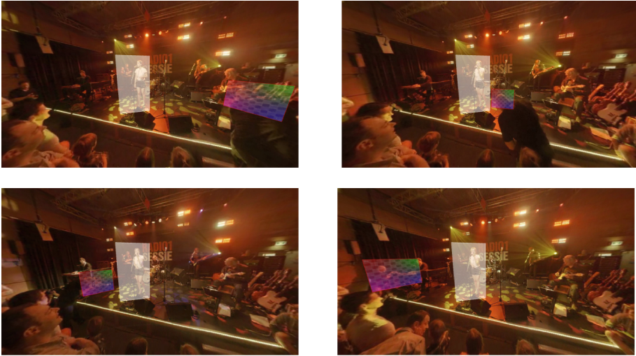
Fig. 3. Illustration of a motion-tracked video overlay . In this specific case, (the head of) an in-video actor was tracked so that an overlay element could be imposed on top of it.
