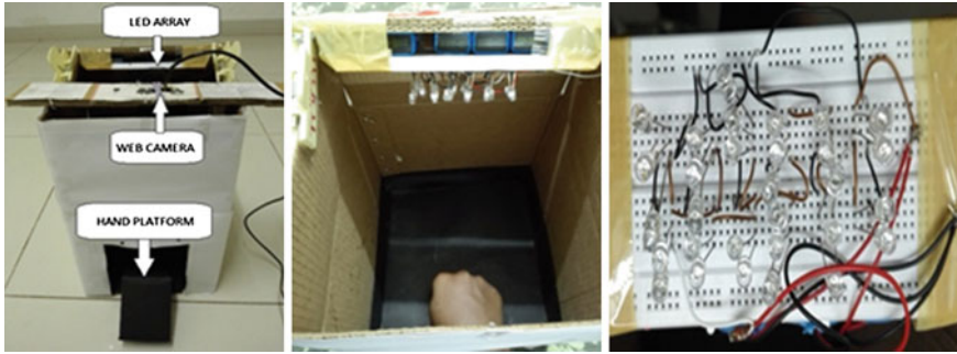
Fig. 1 Palm vein acquisition setup; Top view; Array of LEDs (Left to right)
