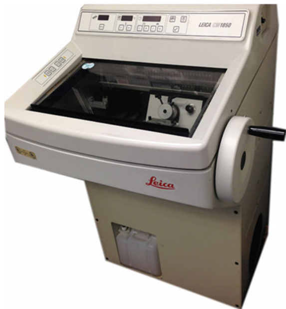
Fig. 6.2 Example of a cryostat manufactured by the company Leica, which is used to cut frozen tissue sections. The temperature inside the chamber can be set using controls on the front panel of the instrument. The rotary handle on the right side of the cryostat is connected to the microtome inside: by rotating the handle clockwise, the tissue block on the microtome moves against the blade, which cuts a tissue section from the frozen tissue block
