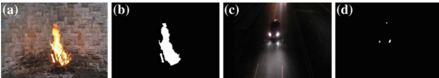
Fig. 2 Foreground images of moving flame and moving vehicle lighting using background subtraction and statistical color model. a Flame image. b Foreground image of flame. c Vehicle lighting image. d Foreground image of moving vehicle lighting
