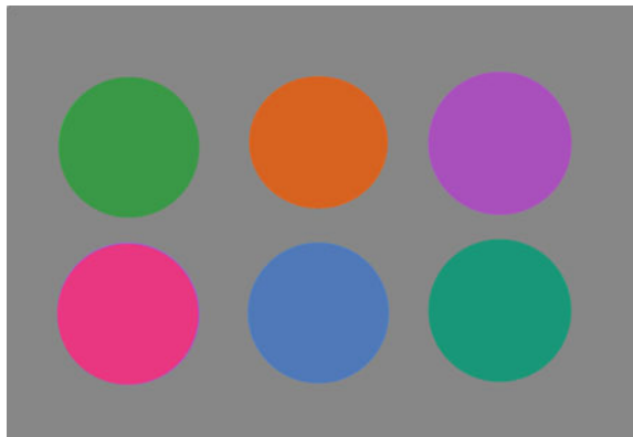
Fig. 58.1 Examples of the Helmholtz–Kohlrausch effect. All circles have the same colorimetric lightness values as the gray surround
