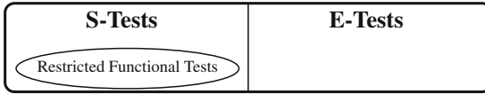
Fig. 3. S-tests, whose purpose is to refute the hypothesis that a system satisfies its specification, include restricted functional tests, which apply to the functionalities the system must offer. E-tests, in contrast, attempt to violate an environmental assumption in an adversarial environment.
