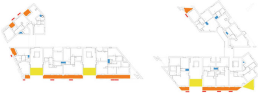
Fig. 60.10 Building plan with passive solar systems. Yellow : common six-story sunspaces that provide preheated air for apartments in winter; orange : private single-floor sunspaces for each apartment; orange : Trombe–Michel walls that support the private sunspaces; blue : ventilation tower that distributes air from sunspaces and from underground slab
