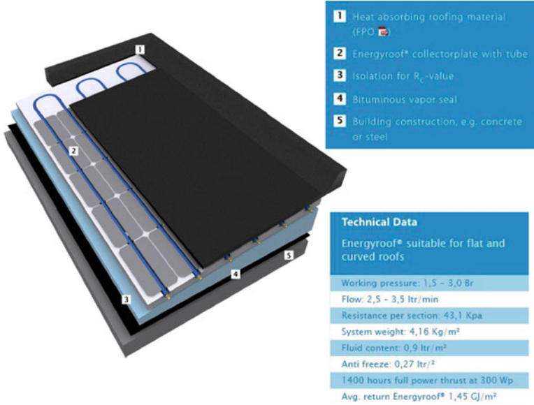
Fig. 5.6 Detail of different layers of energy roof
