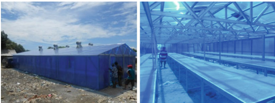
Fig. 65.1 External view (left) and interior of hybrid solar–wind dryer showing racks covered with fishing net
