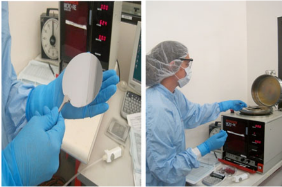
Fig. 15.2 Clean room microengineer. Left: An example silicon wafer. Right: Substrates undergoing surface activation using clean room instrumentation
