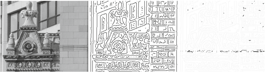
Fig. 6. A fragment from the Wrigley image (original picture on the left) with the sequential program’s traced edge output (middle) and spurious edges rendered by the parallelized version at the lowest fidelity value of 1% (right).
