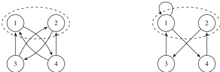
Fig. 2 On the left graph P is periodic and G' is aperiodic. On the right graph P is aperiodic and G' is periodic
