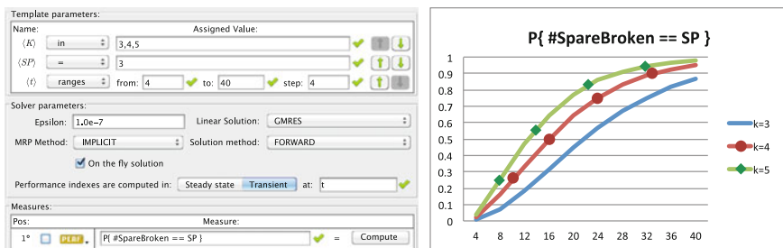
Fig. 9 Distribution of the time for consuming all spares of machine M_2 for a varying number of parts
