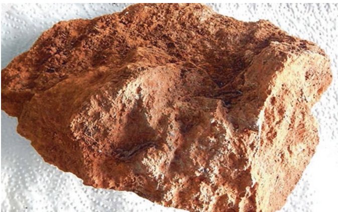
Fig. 1 Gibbsite, \text{Al}(\text{OH})_3 , an ore of aluminium, formed on the surface of Miocene Limestone (Jamaica). Each small circle in the background is 1 mm in diameter. Photo Dwight Rose, Northern Caribbean University
