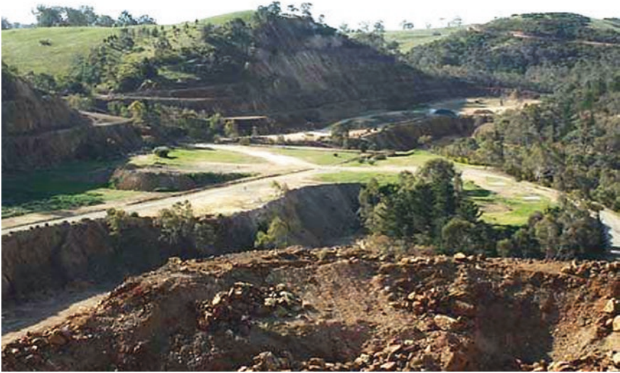
Fig. 10 Brukungu Mine, South Australia. Waste rock heaped along a creek bank remains un-vegetated. Rainfall maximum here is unimodal (winter only). Comparing this result with that of the more intense bimodal rainfall regime of a similar pyrites mine in the mountainous Trade Wind region of Dominican Republic could reveal greater environmental impacts. Source South Australia Government Documents at: www.minerals.dmitre.sa.gov.au
