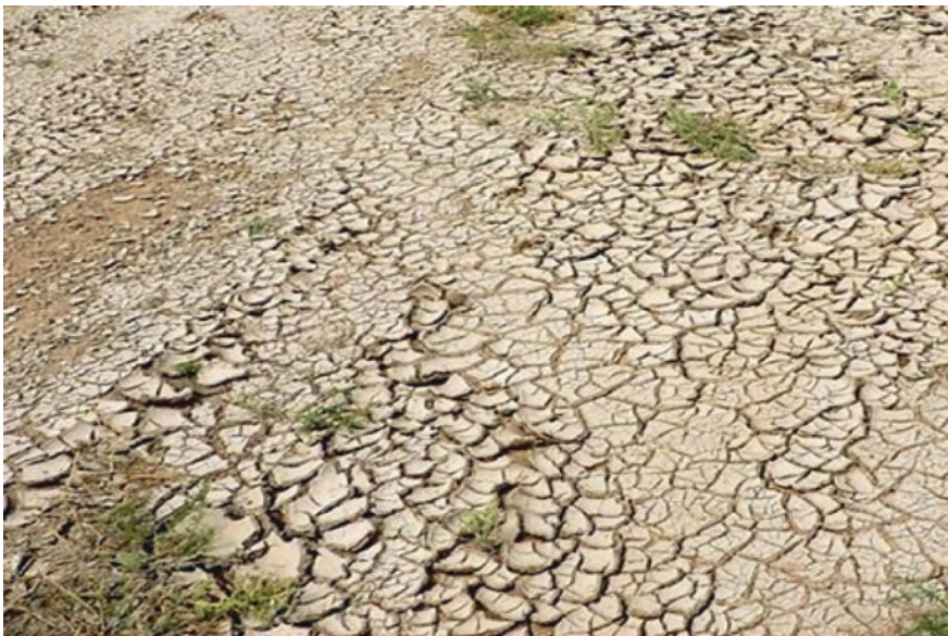
Fig. 1 Surface crusting of a sodic soil. The soil attains high strength which restricts root penetration. Source usgs.gov
