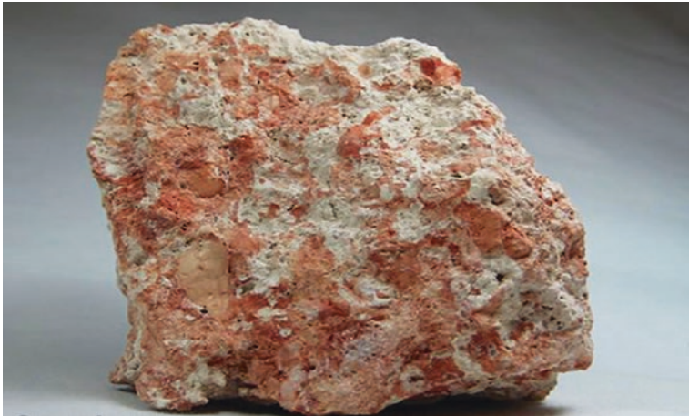
Fig. 6 Guyana bauxite is often in the form of a pink rock, contrasting with the soft, earthy, easily-worked Jamaican ore. Mine capping therefore is more costly and logistically and edaphically more difficult in Guyana. Source Demarara Bauxite Company (DEMBA)
