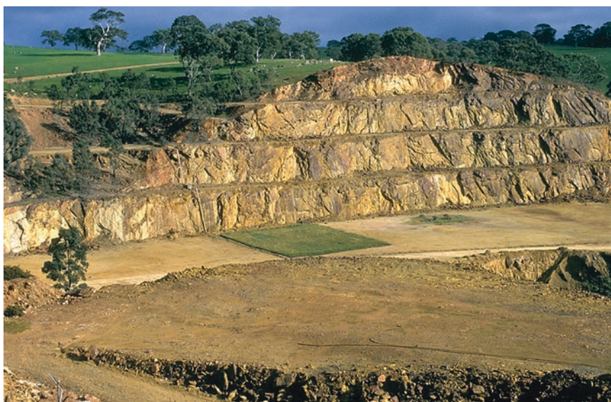
Fig. 1 The step-like pattern of open-pit sulfidic mines exposes pyrite to oxidation by a factor of at least 2:1. Source: QGRM (2002)
