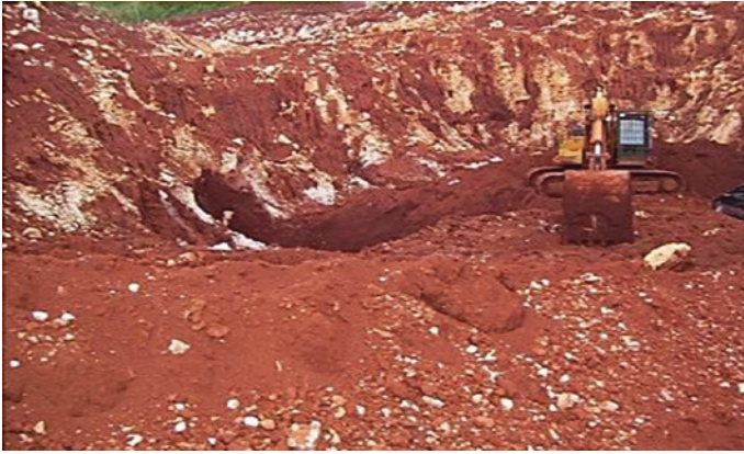
Fig. 1 In this active karst bauxite mine pit, the apparent differentiation between top-soil horizons and sub-soil zone is not easily observed or detected. This can cause inadvertent mixing of top-soil with sub-soil. Source: usgs.gov
