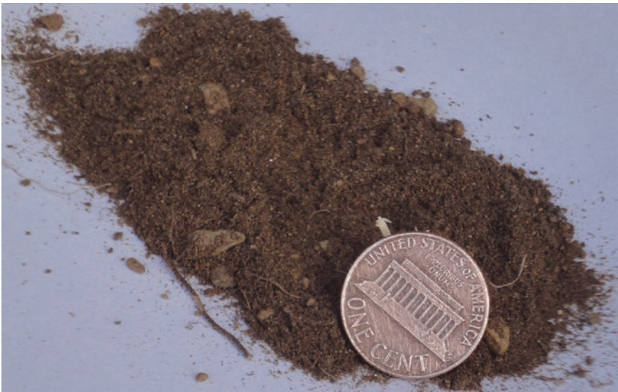
Fig. 13 Leachate residue ( \text{CASO}_4 + contaminants) intermixed with sewage sludge incubated with phyto-organics. Note improved aggregation
