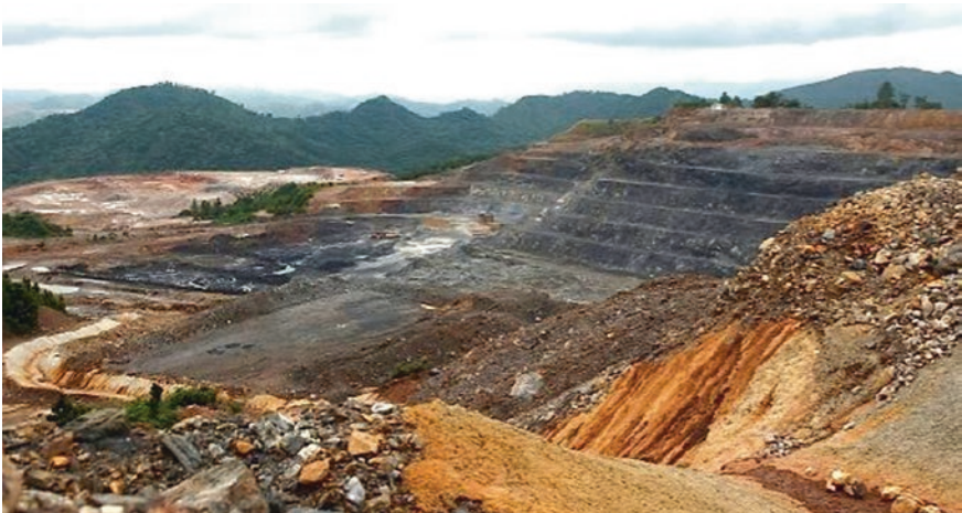
Fig. 11 Pueblo Viejo gold mine, Dominican Republic. Note staining at right by leachate from atmospheric exposure of pyritic waste rocks. Heavy, frequent cumulonimbus clouds seen at top of photo signify a more humid climate compared to that of South Australia (see Fig. 9), indicating more moisture for sulfuric acid generation in the ground. Source Barrick Gold Corporation
