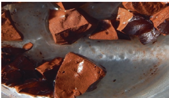
Fig. 9 Dried gypsum-treated red mud waste (GRMW) had no observable reaction with water, retaining its stability even after many weeks. Scale is supplied by 1-mm-diameter indented circles in the background
