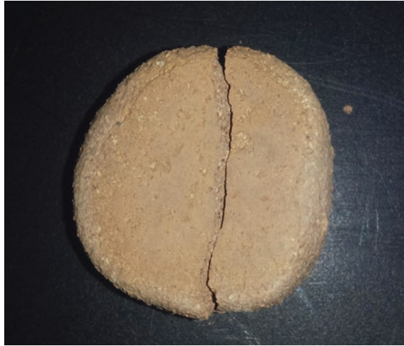
Fig. 2 Failure of sample in a direction of the applied load using the Brazilian Indirect Tensile Strength Test. All samples failed in this direction
