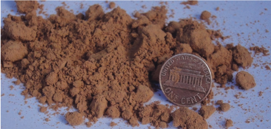
Fig. 12 Leachate residue ( \text{CASO}_4 + contaminants) at Brukungu Mines, South Australia. Note structure-less consistency
