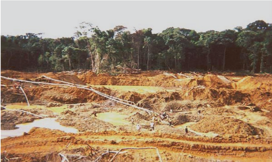
Fig. 7 A gold mine excavation in Guyana. The uneven, pock-marked surface with pools at varying levels presents difficulties for subsequent mine-capping operations. Source Barrick Gold 2012
