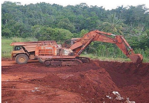
Fig. 8 Scooping of overburden causing mixing of top-soil with sub-soil unintentionally dilutes the quality of the top-soil. Specially calibrated equipment is required (source: usgs.gov)
