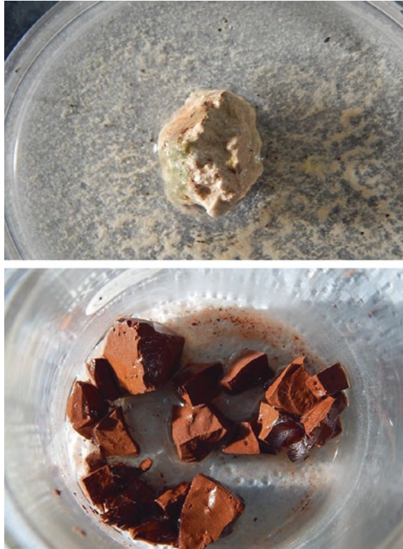
Fig. 6 a Slaking of rocks. The mass of material slaked and removed from the soft limestone (whitish, located in laboratory watch glass) by the water was 5 times that removed from lithified red mud (G). b Lithified red mud (G)
