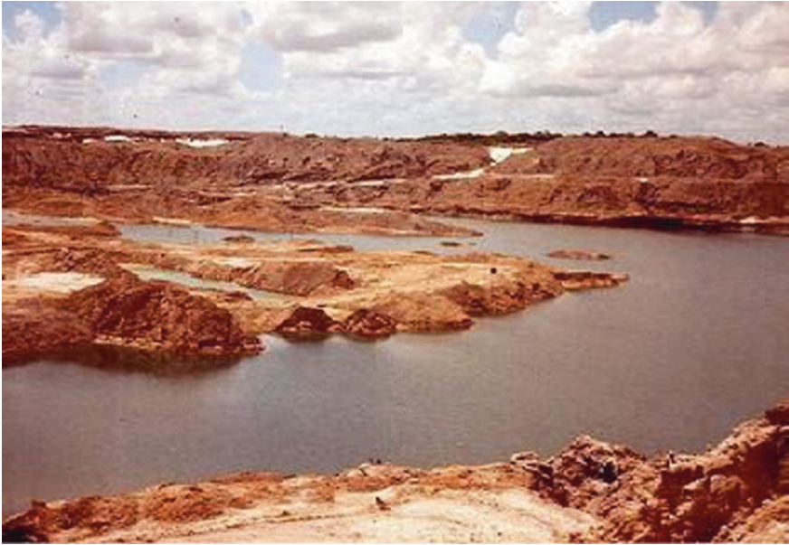
Fig. 5 A Guyana bauxite mine. Bauxite is located much more deeply; >3-fold the depth of Jamaica mines. Note the deep lakes formed in the mined out locations, thereby presenting almost insurmountable obstacles to land rehabilitation. Source Demarara Bauxite Company (DEMBA)
