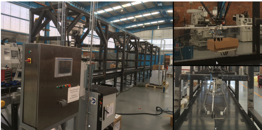
Fig. 7. (a) Automatic recycling line prototype. (b) Suction pad, for materials such as glass, paper or paperboard, and (c) gripper, for materials such as aluminum cans and plastic bottles.
