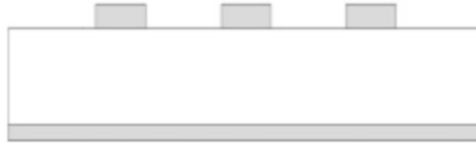
Fig. 3 Three conductor transmission line
