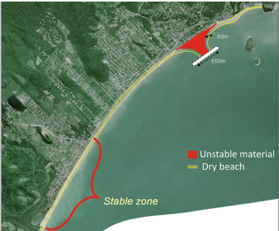
Fig. 2.19 Location of the detached breakwater and predicted equilibrium planform proposed to solve the central beach erosion
