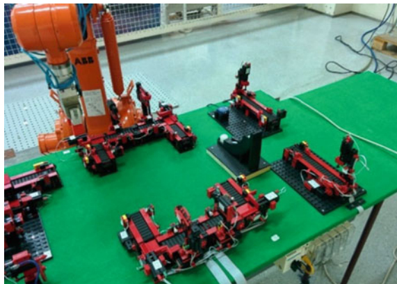
Fig. 4 Layout of the small-scale production system
