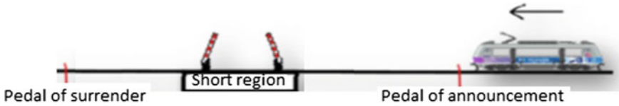
Fig. 1 Principle of functioning of the automated level crossing
