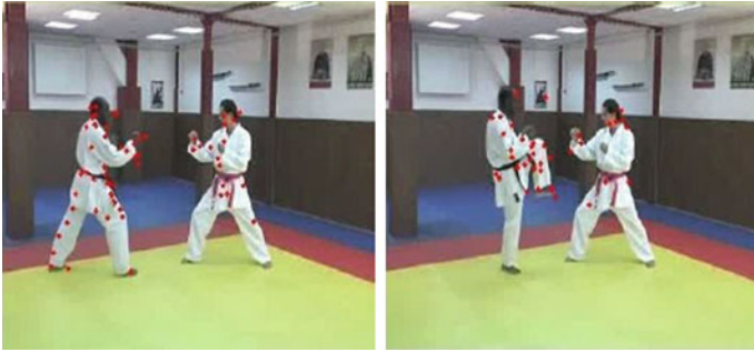
Fig. 4 Examples of clouds of color space-time interest points, in each frame (Image (t = 44)/ Image (t = 45)), we use the parameters ( \sigma_t = 1.5 , k = 0.04 and \sigma_s = 1.5 )
