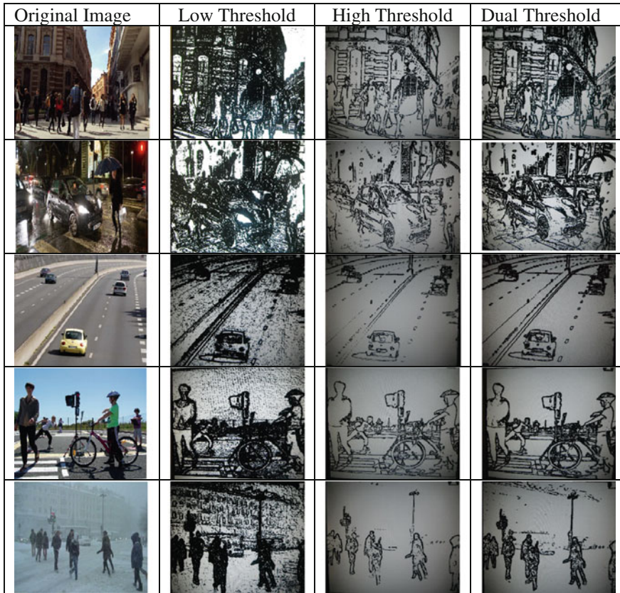
Fig. 4 Results for Sobel edge detection. Original image, low threshold, high threshold, dual threshold
