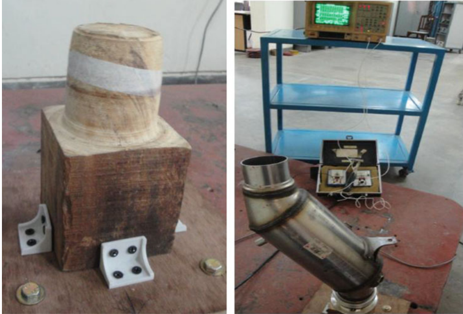
Photo Courtesy IISC: Wooden Fixture ( left ) and converter assembly on the fixture setup ( right )
