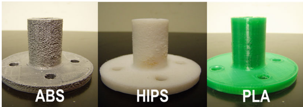
Fig. 17.5 Parts printed up to the top of the accelerometer cavity with manufacturer's suggested settings for different materials
