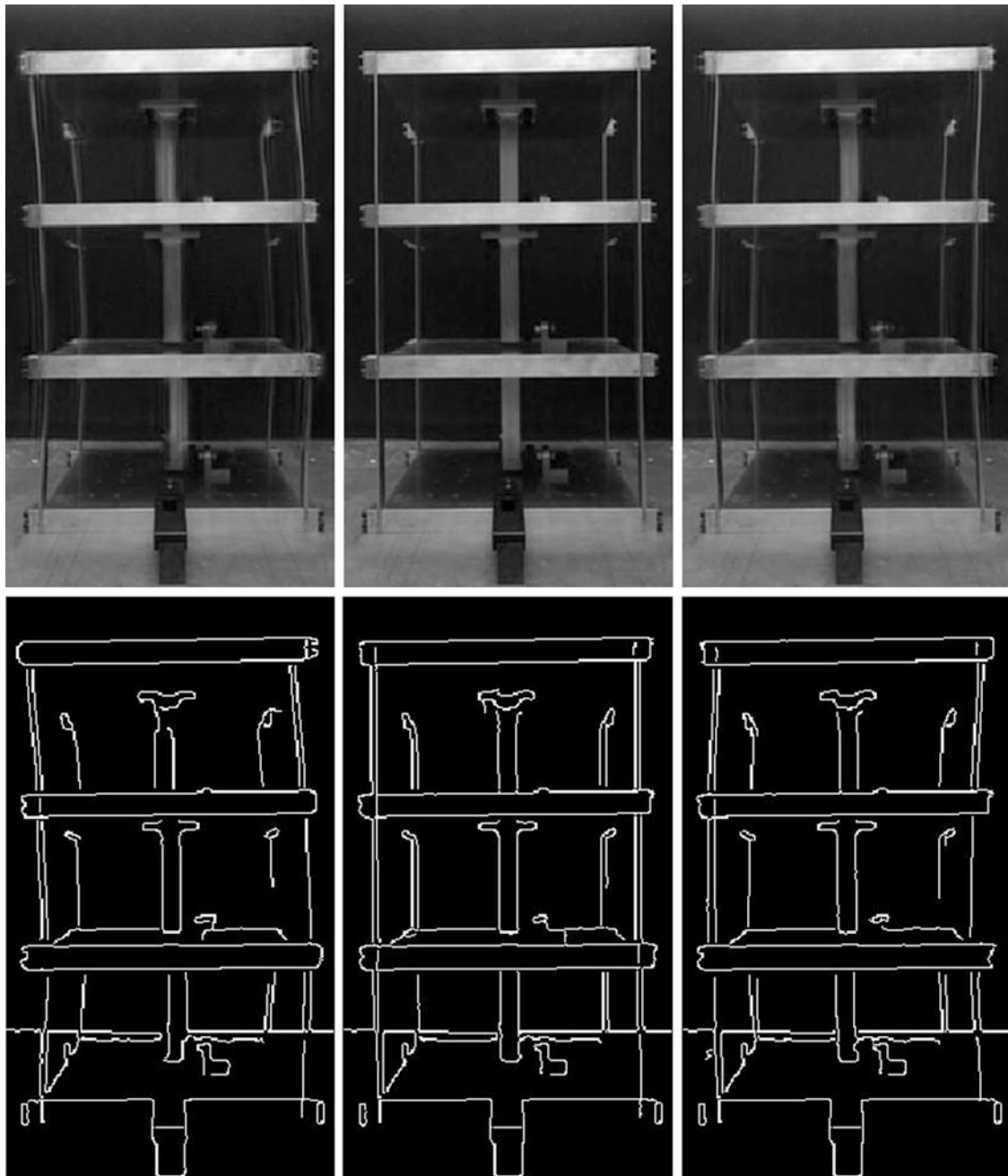
Fig. 32.3 A few frames from the motion magnified video (mode 2) (first row) and their corresponding mode shapes (second row) by conducting the edge detection
