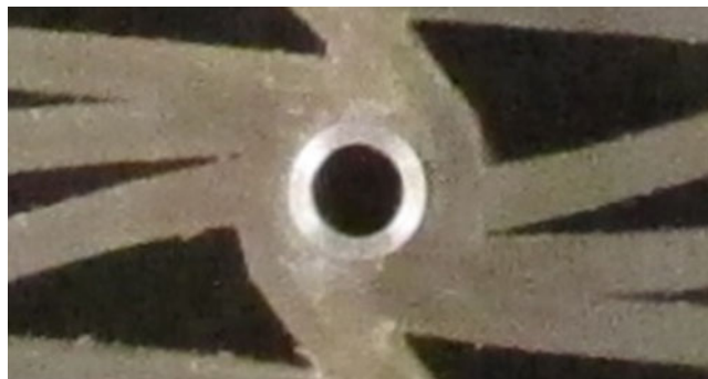
Fig. 16.1 Close up view of annular mass and ligaments
