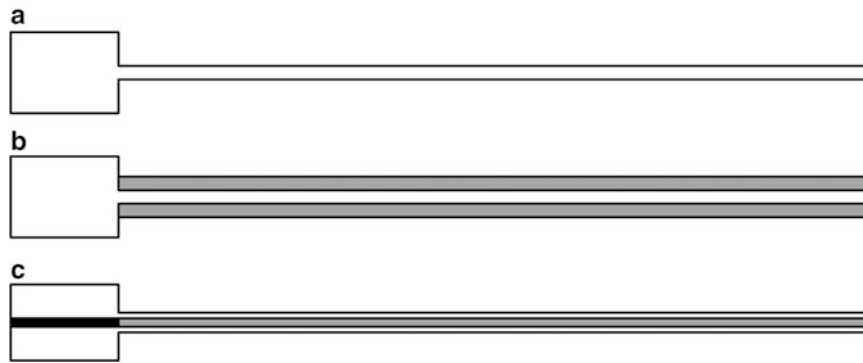
Fig. 15.3 Testing configurations (a) uniform beam, (b) modified Oberst beam, (c) sandwich beam
