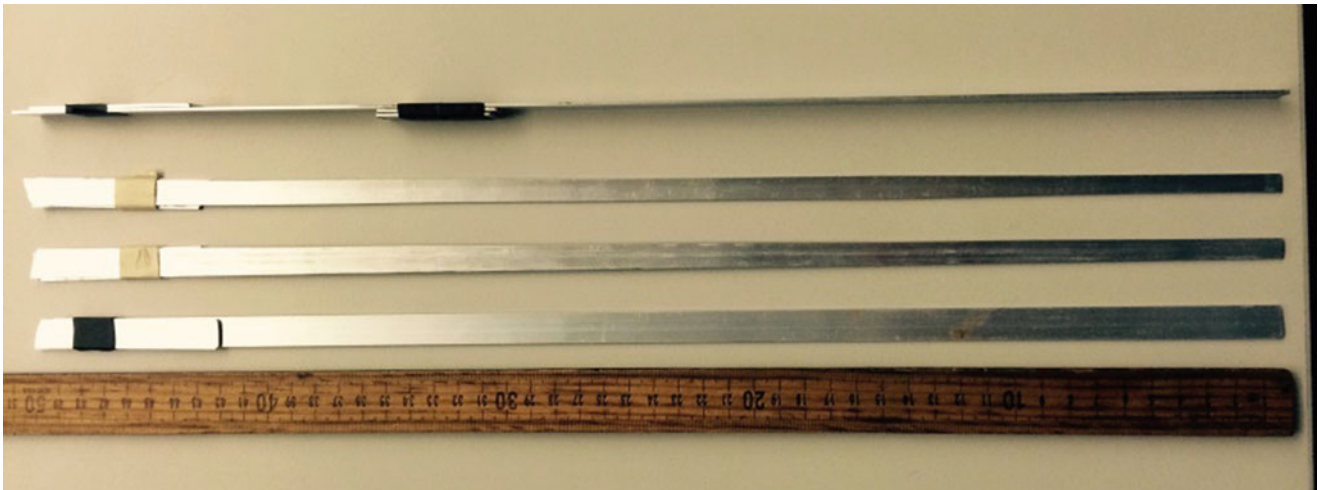
Fig. 11.2 Alterations to beam geometry. From bottom to top we have: regular beam, asymmetric beam, symmetric beam and weighted beam
