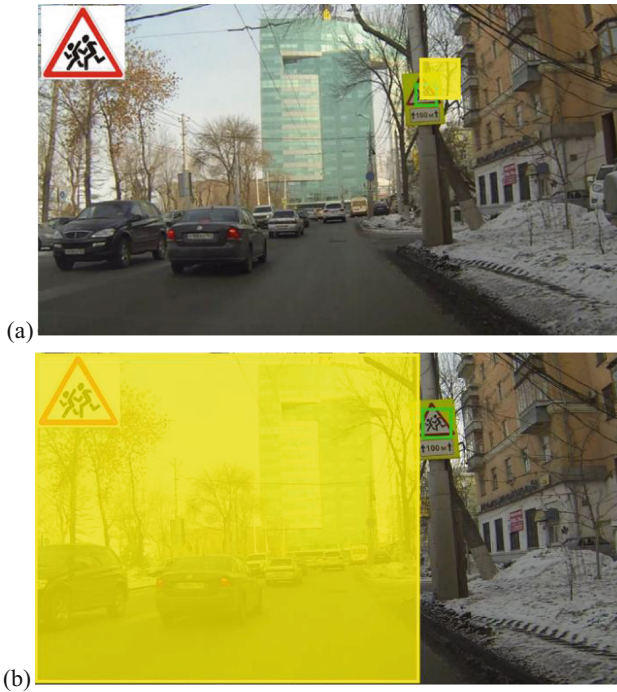
Fig. 11. (a) A frame with marked calculated area of interest for the next frame; (b) The next frame with marked area for searching new objects.
