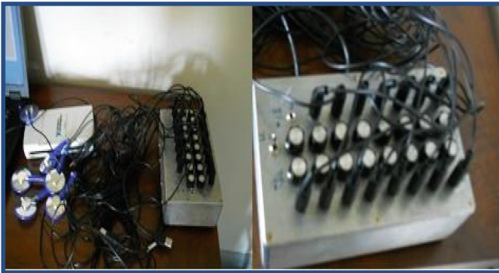
Fig. 3. Multichannel lung sound system, capture of the detailed devices used in the multichannel stethoscope (sensors, I/O box of connexion and DAQ server).
