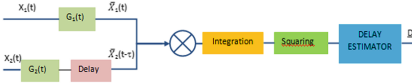
Fig. 6. Received waveforms filtered, delayed, multiplied and integrated for a variety of delays until peak output is obtained.
