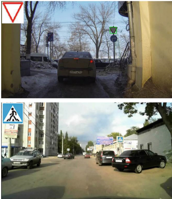
Fig. 10. Frames from a video sequence with detected and classified traffic signs.
