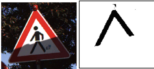
Fig. 2. Example of color extraction in RGB (Color figure online).
