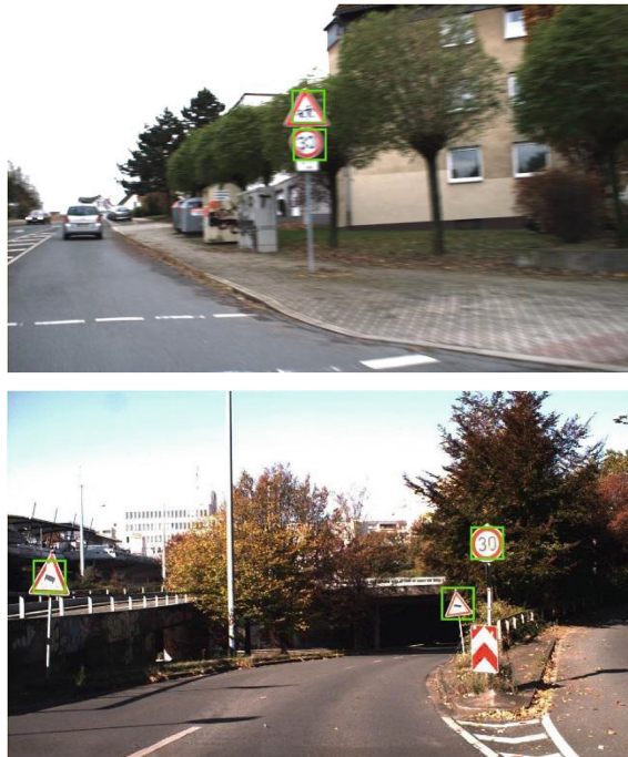
Fig. 8. Traffic signs detection in images from the GTSDDB dataset.
