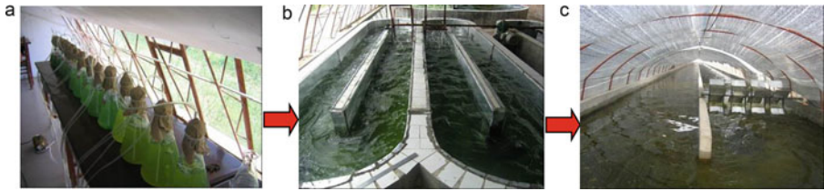
Fig. 24.4 Mass cultivation procedure and equipment used for cyanobacteria ( Microcoleus vaginatus ) culture in Inner Mongolia. (a) The first grade mass culture of isolated cyanobacteria in flasks; (b) Small raceway culture ponds for further mass culture; (c) A large raceway culture pond. (Photo by Weibo Wang)
