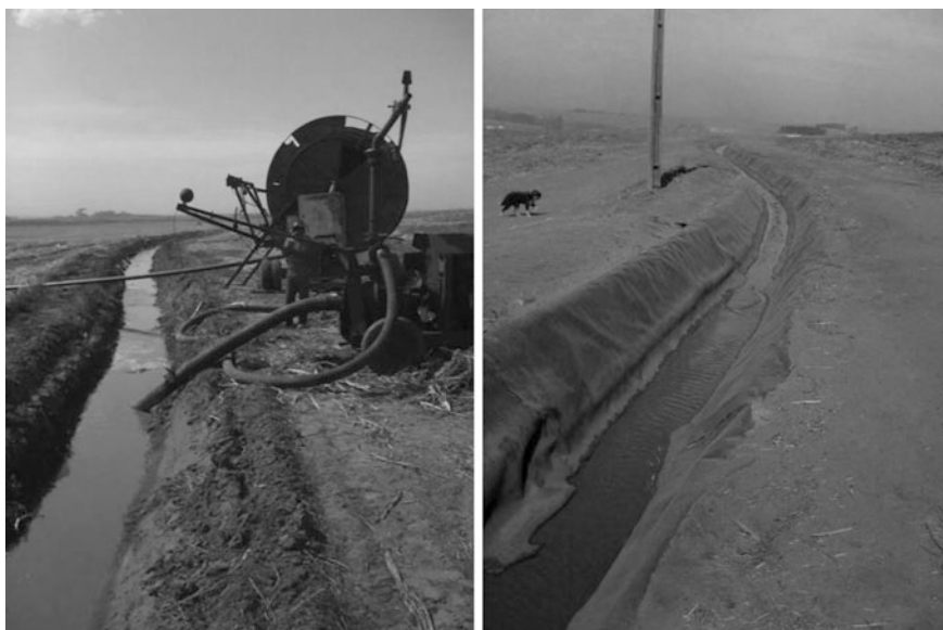
Fig. 5 Channels for the distribution of vinasse along the field ( left ) and coated channel in an ethanol and sugar industry located in São Paulo, Brazil. Source The authors
