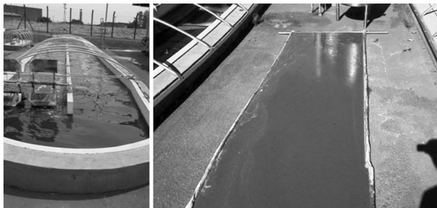
Fig. 10 10 m 3 raceway of Spirulina platensis biomass production in 50 % vinasse medium (left) and the filtered biomass drying in the sun (right). Source The authors
