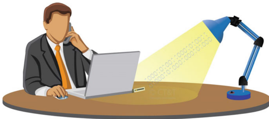
Fig. 1.6 A VLC-enabled hot spot composed of a USB dongle receiver and a desk lamp based VLC transmitter
