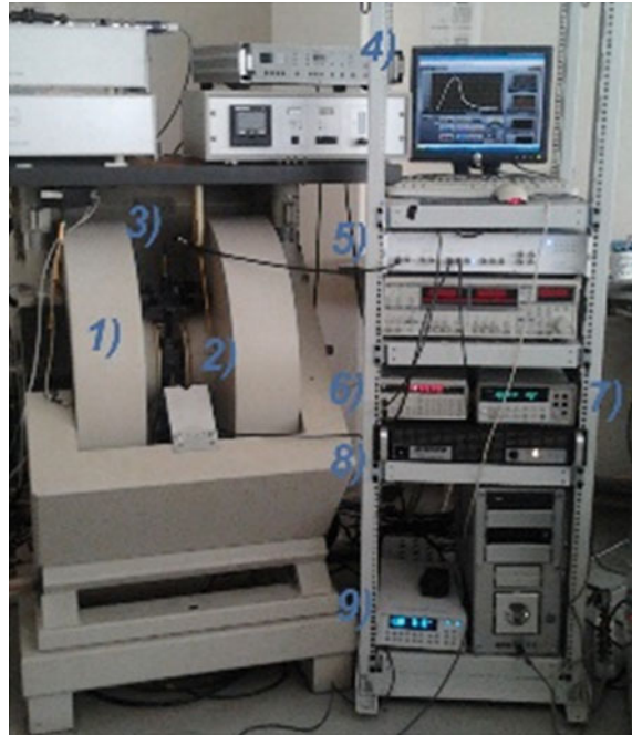
Fig. 7.2 Photo of the setup used in the ME measurements. The labeled components are: 1) electromagnet; 2) box containing the Helmholtz coil; 3) sample support and goniometer; 4) PC; 5) lock-in amplifier; 6) function generator; 7) multimeter (ammeter/voltmeter); 8) power amplifier; 9) gaussmeter
