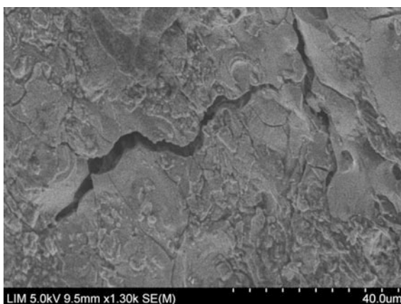
Fig. 14.16 Aspect of surface obtained by hybrid electrochemical discharge drilling of small diameter holes (workpiece made of high speed steel, tool electrode diameter d_{TE} = 0.5 mm, aqueous solution of soluble sodium silicate, electrolyte density \delta = 1.20 g/cm 3 , U = 45 V, C = 840 \mu F, image obtained by means of scanning electron microscope Hitachi S-4800) (Coteață [16])
