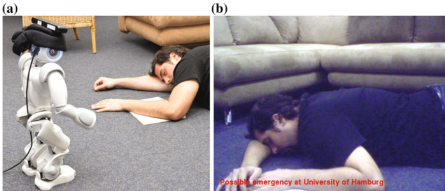
Fig. 10 Fall detection scenario: In case a fall event is detected by the system, the Nao will approach the fallen person (a) and take a picture of the scene (b)
