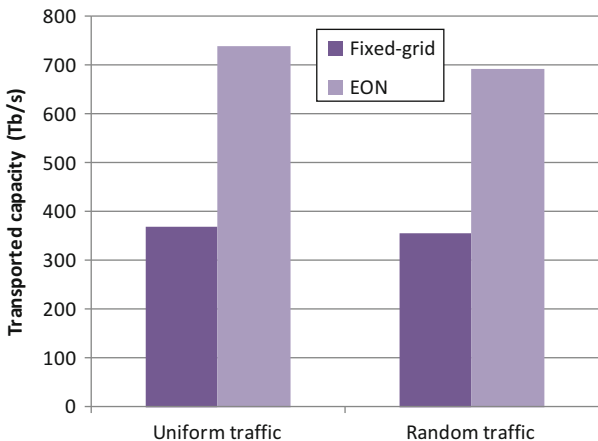
Fig. 3.6 Maximum transported capacity obtained for each scenario for the fixed-grid and EON case over the 22-node BT core network
