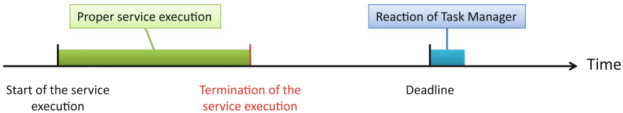
Fig. 10 Time diagram of service a failure without notification
