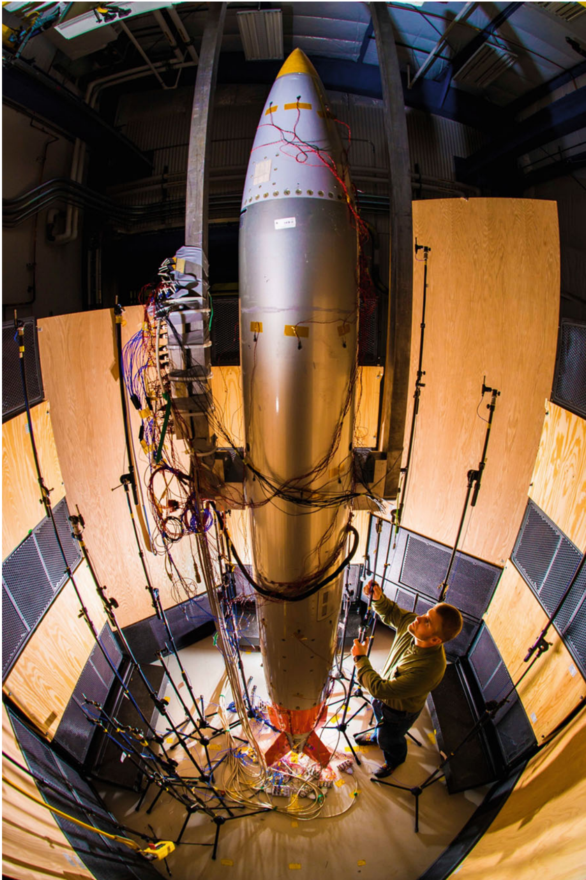
Fig. 4.3 Acoustic “Truth” test setup
