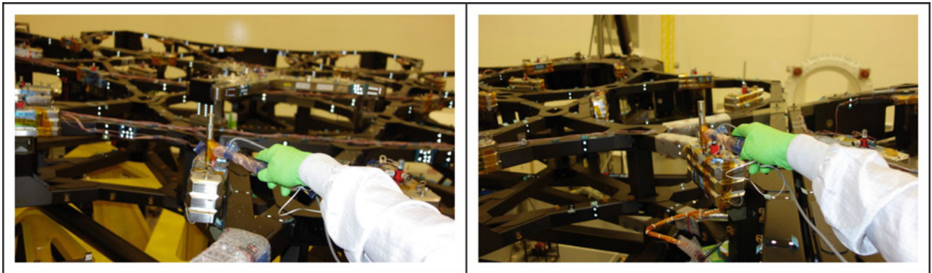
Fig. 10.12 Primary mirror mass simulator impacts—example photos of two locations
