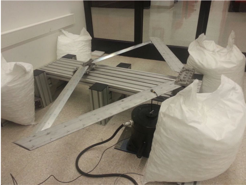
Fig. 9.17 Test setup for shaker test of the Design Point 2
