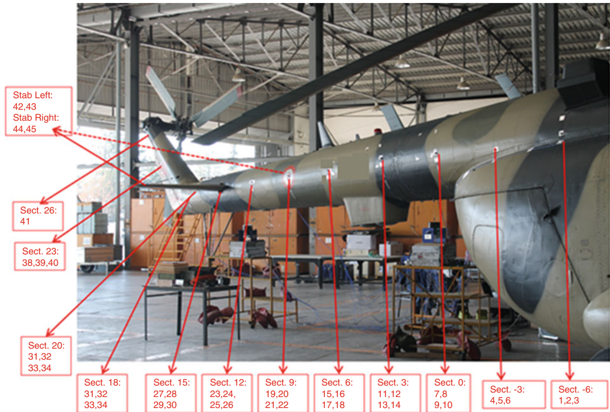
Fig. 12.8 Modal test setup for the helicopter tail boom
