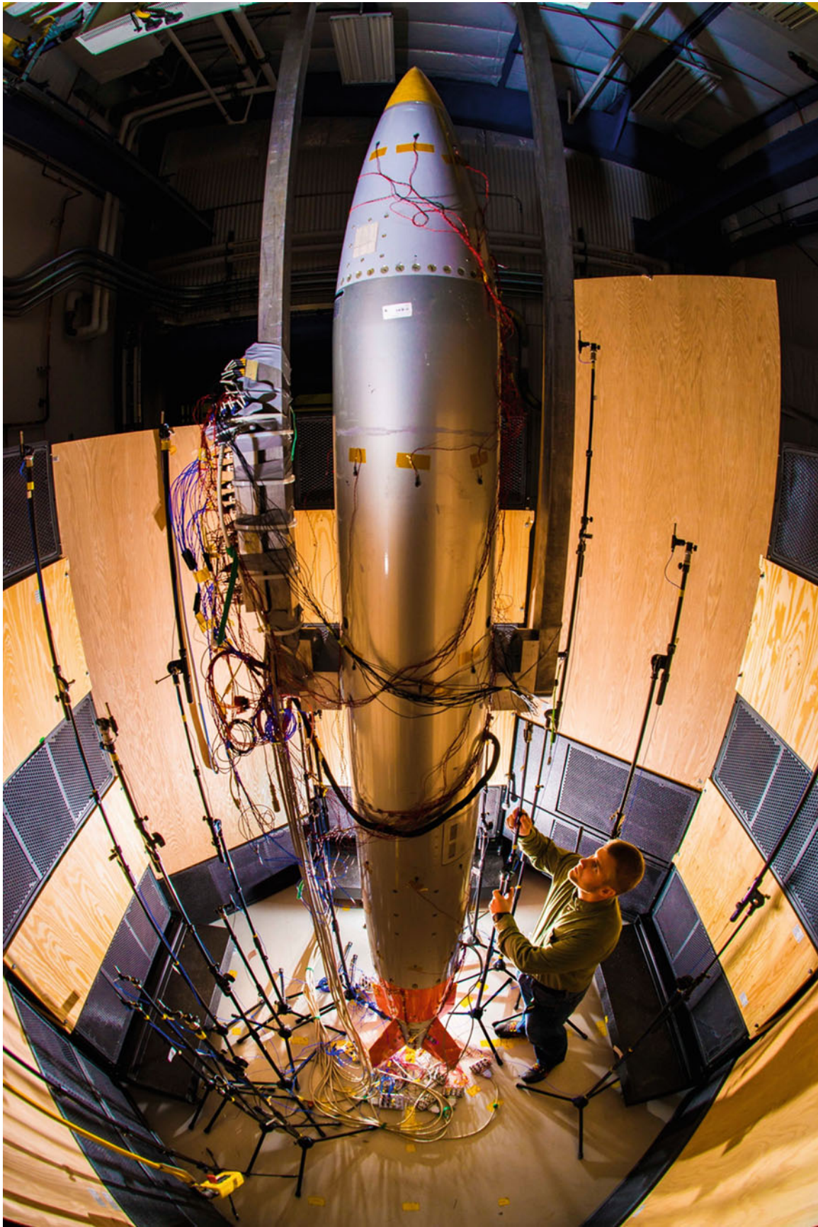
Fig. 4.3 Acoustic “Truth” test setup
