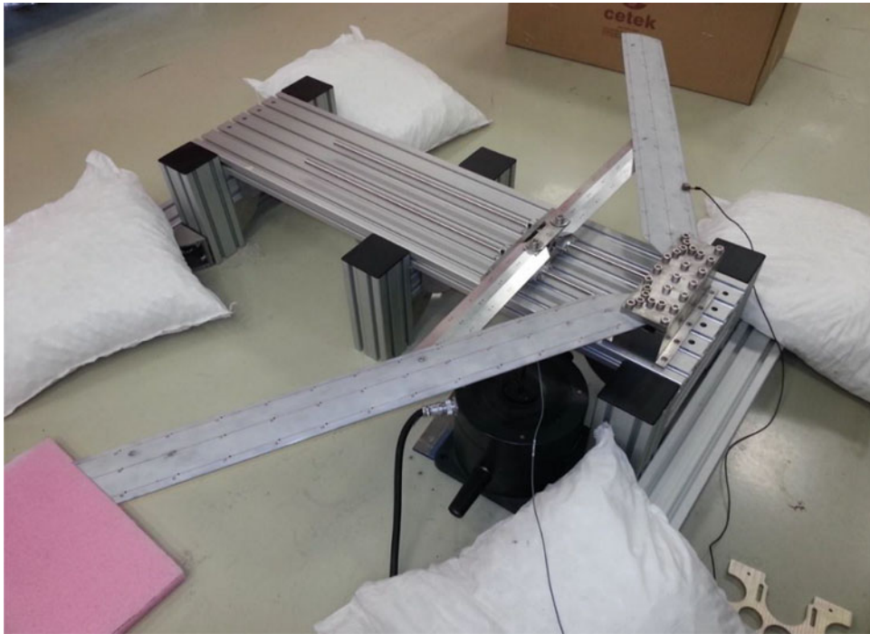
Fig. 9.12 Test setup for shaker test of the Design Point 1
