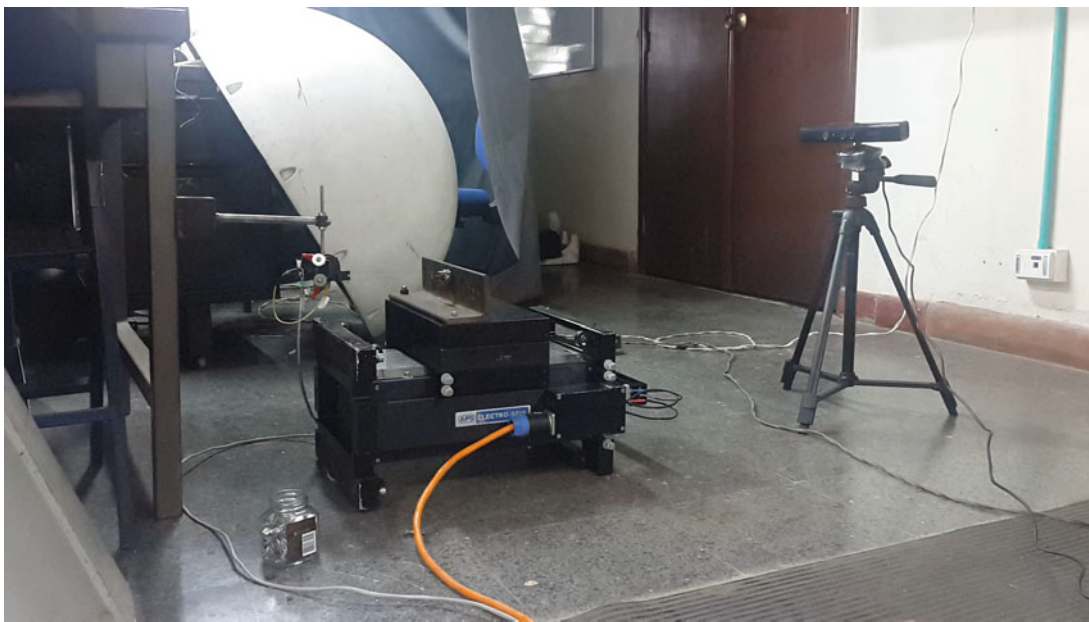
Fig. 2.4 Experimental setup for dynamic displacement approach
